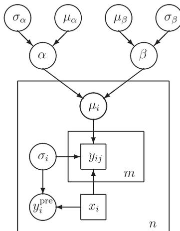
Fig. 1. The DAG of the hierarchical Bayesian model for estimating S-N curve or P-S-N curves. The arrows represent dependencies of variables, which are assumed to be independent conditional on each level. These nodes with fixed quantities in the analysis are represented by rectangles, while unobserved random variables are represented by circles.
