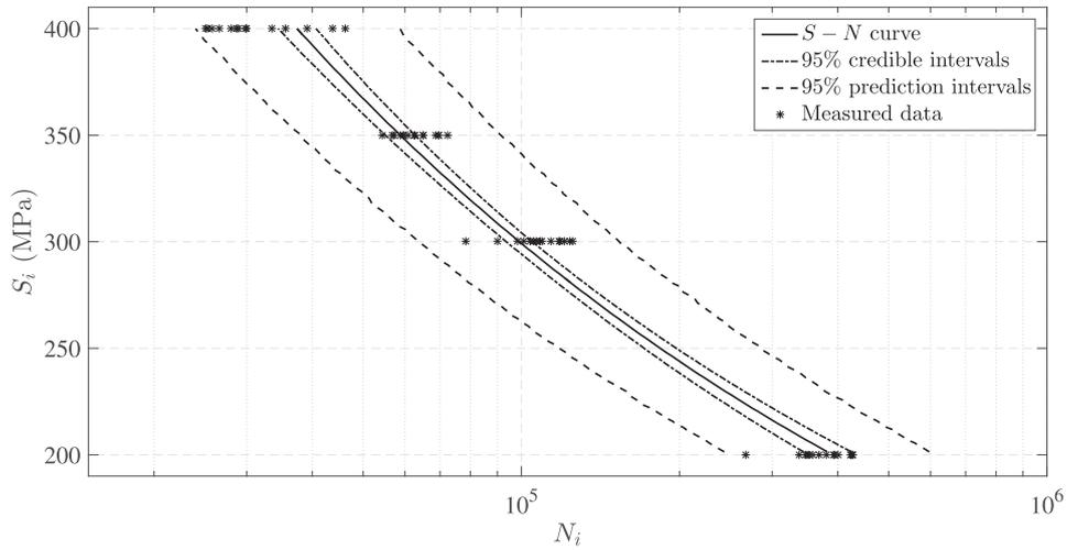
Fig. 3. The  $S-N$  curve fitting and  $P-S-N$  curves estimation, with 97.5% survival probability or 95% prediction intervals, in Example 1.
