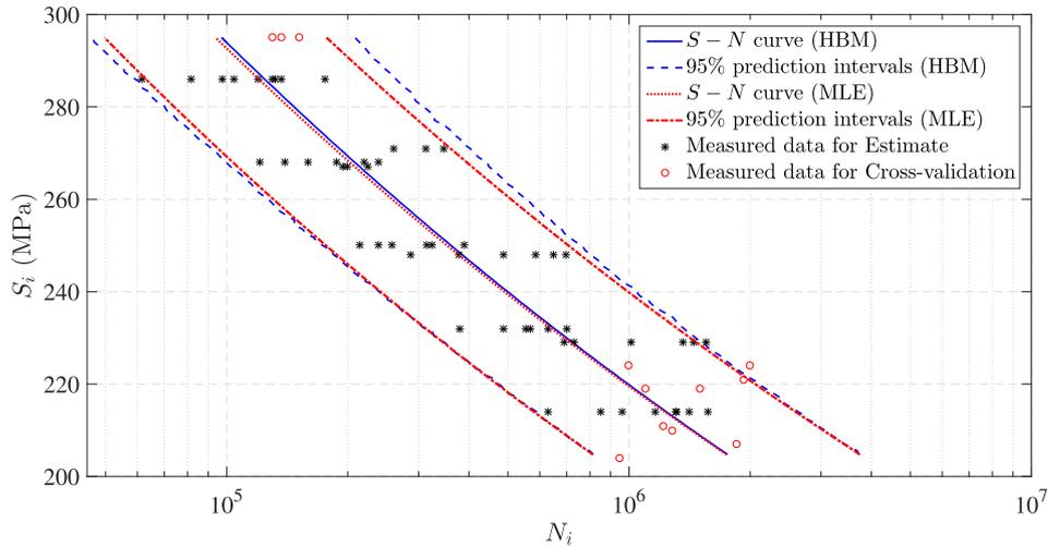
Fig. 8. A comparison of the hierarchical Bayesian model (Case 1) and MLE to estimate  $S-N$  curve and  $P-S-N$  curves in Example 2.
