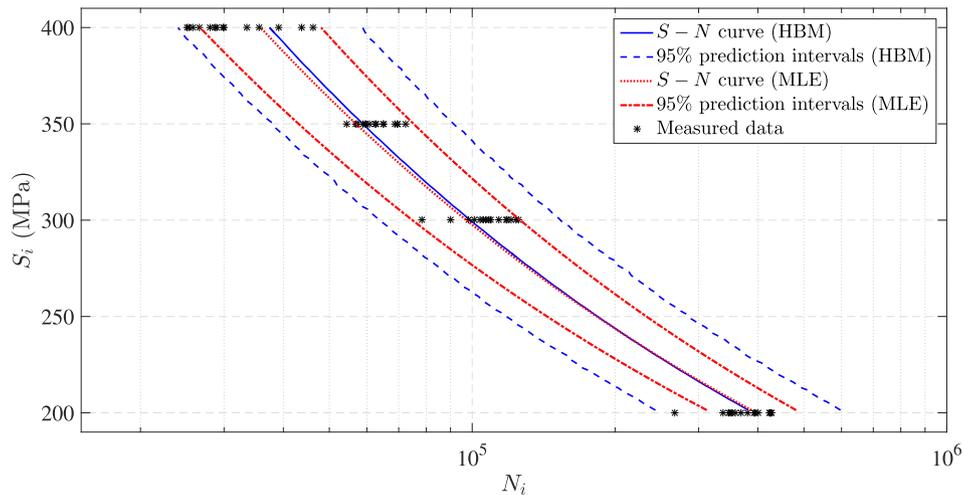
Fig. 7. A comparison of the hierarchical Bayesian model (Case 1) and MLE to estimate S-N curve and P-S-N curves in Example 1.
