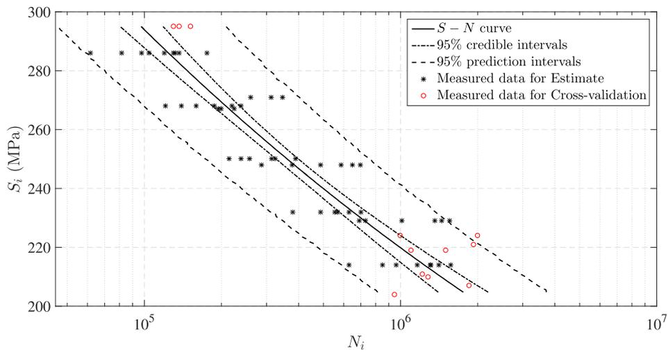
Fig. 4. The  $S-N$  curve fitting and  $P-S-N$  curves estimation, with 97.5% survival probability or 95% prediction intervals, in Example 2.
