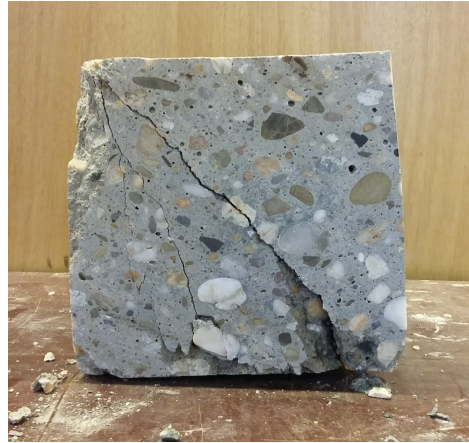
Figure 5-21: Concrete compressive strength test: crack pattern.
