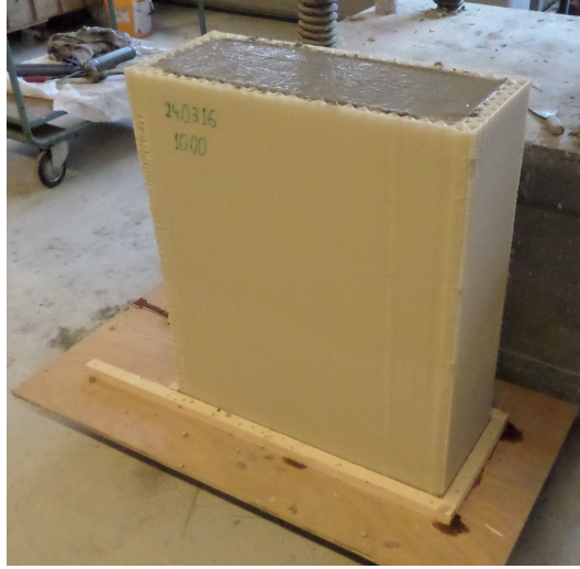
Figure 5-20: Casting of a built-up mould.
