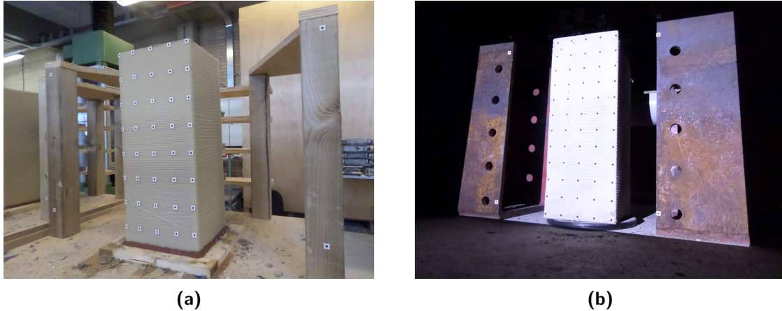
Figure I-1: Photogrammetry setups. (a) before demoulding, glued dots (b) after demoulding, projected dots.
