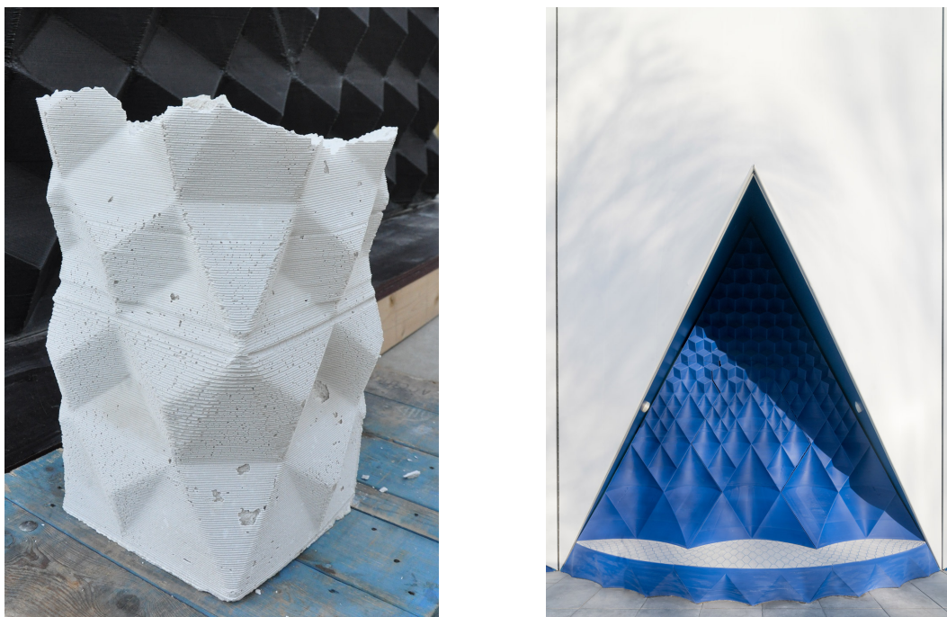
Figure 2-6: 3D Print Canal House: application of concrete. Left: casting test on site. Right: Bench in the Europe Building in Amsterdam (DUS Architects, 2016).
