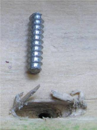
Figure 4.11 –Failure of the fastener
