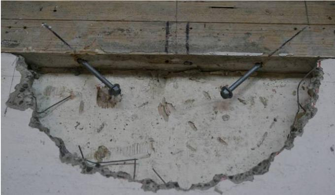
Figure 4.3 – Timber-to-concrete connection with screws under a 45° angle
