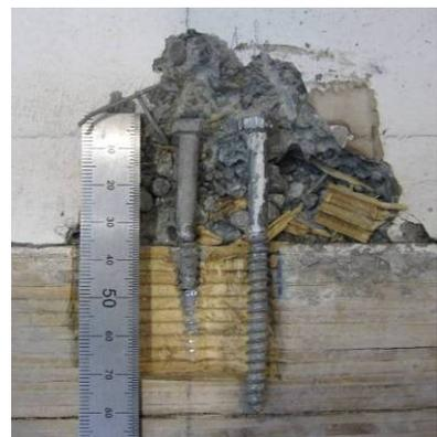
Figure 4.1 – Double yielding in the fastener [Le Heux, 2008]
