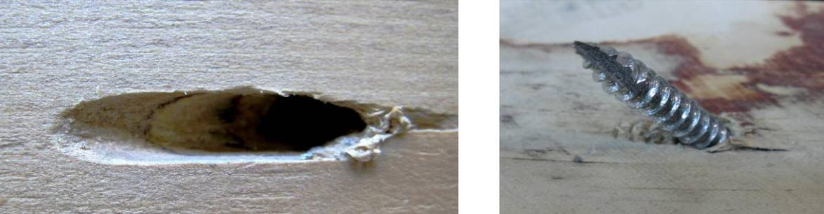
Figure 4.15 – Failure in the timber frame and the screw still fixed to the joist
