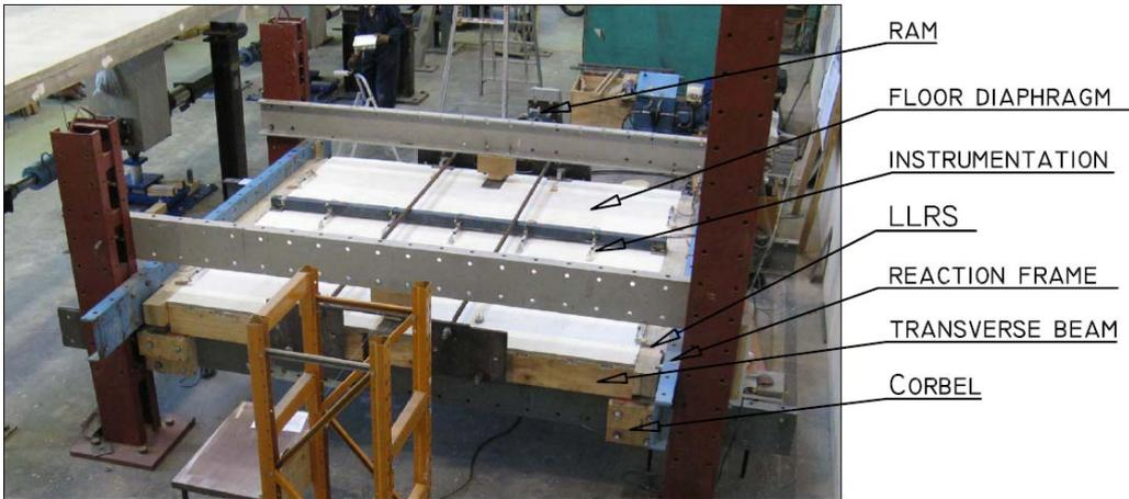
Figure 3.1 – Test setup in the laboratory
