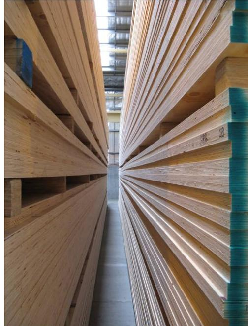
Figure 3.5 – Stack of LVL panels
