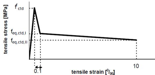
Stress strain diagram 4-points bending test
