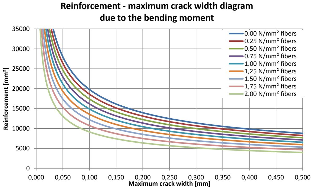
In this figure the reinforcement over the maximum crack width is plotted. In this graph the reduction of the reinforcement and the maximum crack width can be seen if steel fibres are added.
