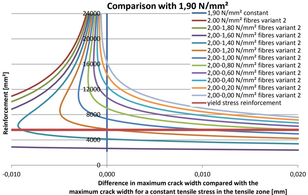
8-7 Comparison post-cracking behaviour with 1,90 N/mm<sup>2</sup>
