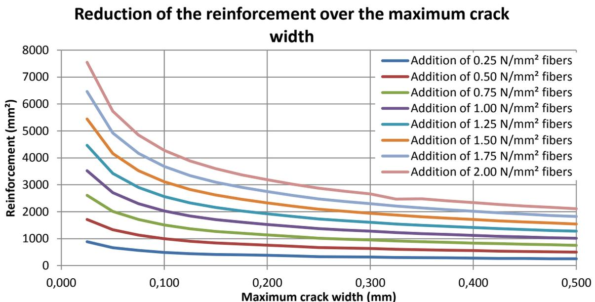
6-4 Reduction of the reinforcement over the maximum crack width
