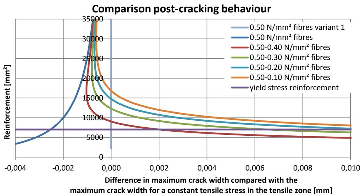
8-2 Comparison post-cracking behaviour with  $\sigma_f=0.50 \text{ N/mm}^2$
