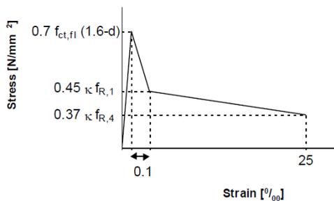
Stress strain diagram Rilem method
