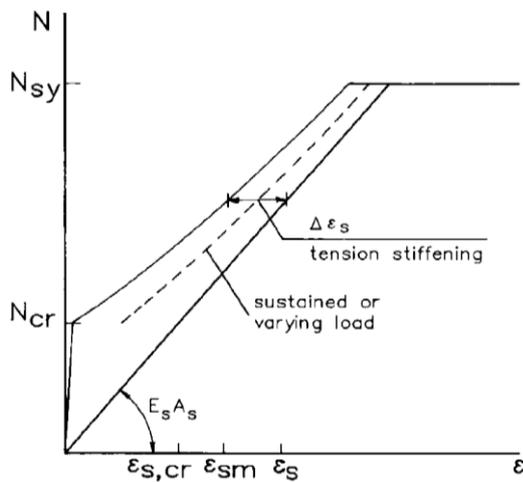
3-7 Tensile force – strain curve of a reinforced tensile member by Leonhardt
