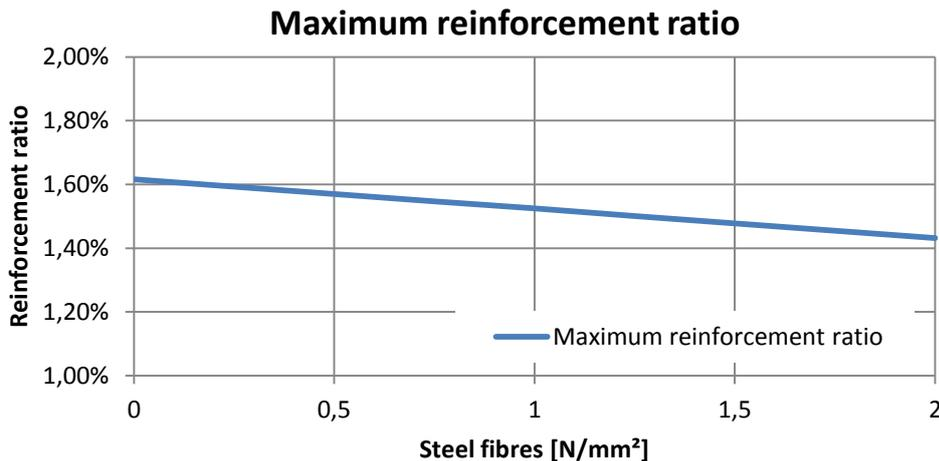
4-3 Maximum reinforcement ratio over the total width of the bridge (2.5m)
