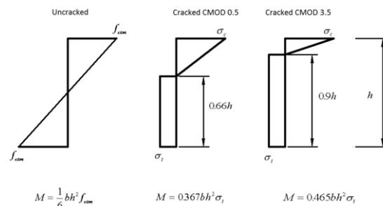
Cross sections of uncracked concrete, a CMOD of 0.5 mm and a CMOD of 3.5 mm
