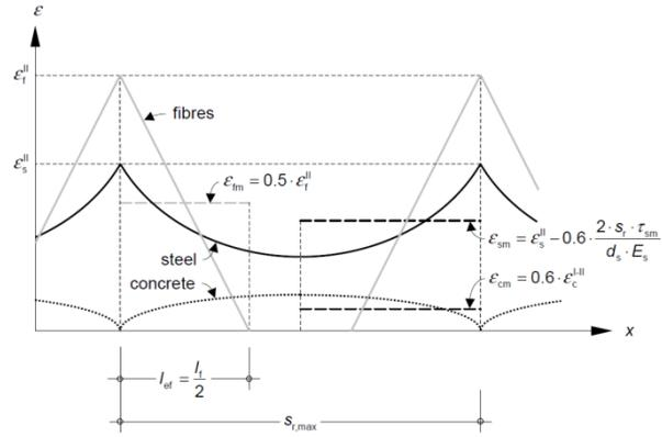
Steel and concrete strain diagram close to a crack in the crack stabilized stage
