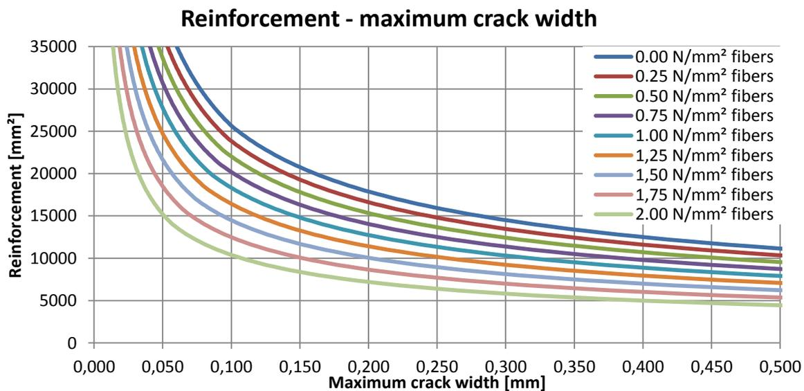
7-8 Reinforcement - maximum crack width all loads
