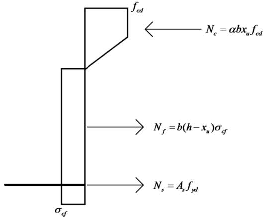
4-2 Cross section of steel fibre reinforced concrete in the Ultimate Limit State
