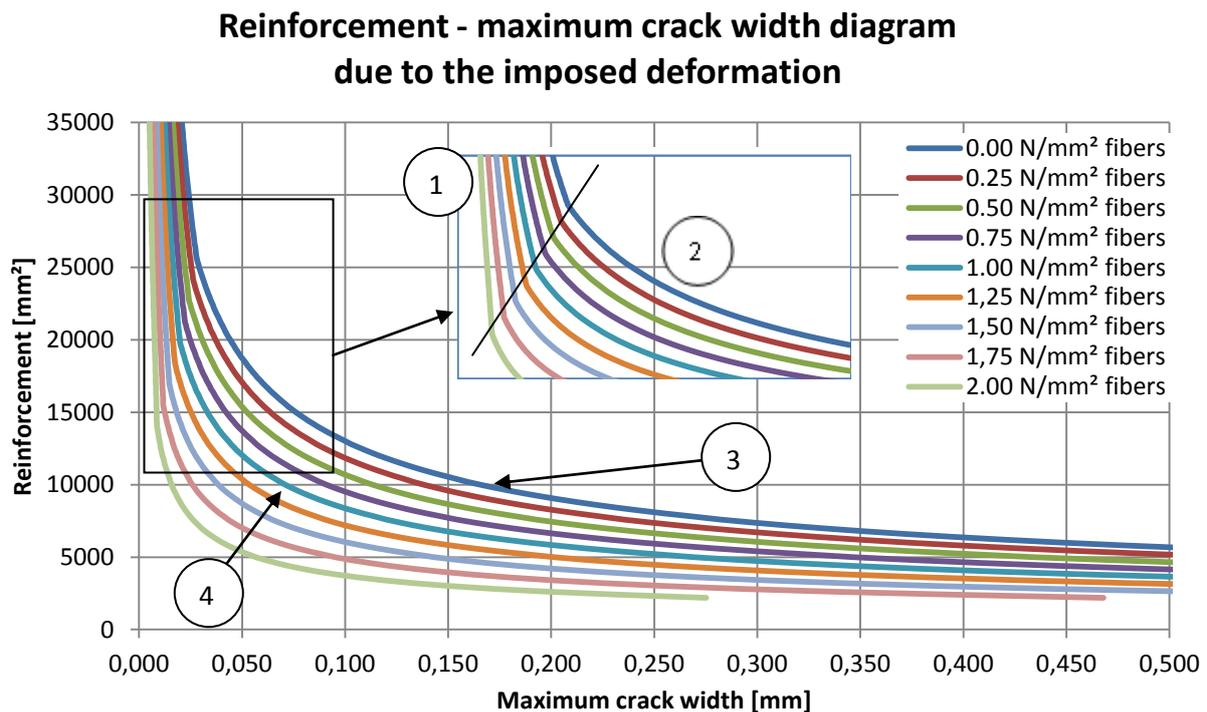
7-4 Reinforcement - maximum crack width due to imposed deformation
