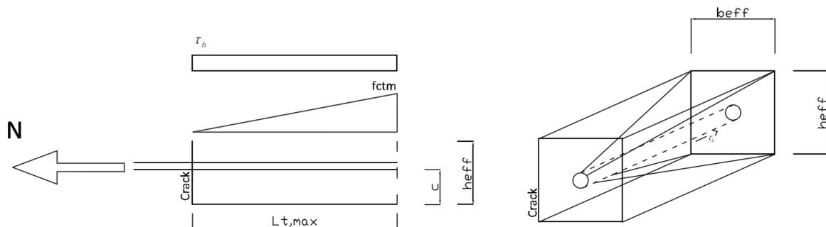
3-9 Introduction of the tensile force in a concrete beam
