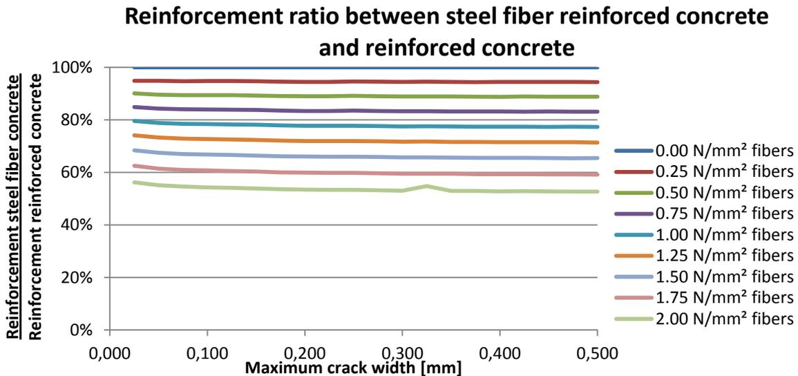
6-5 Reinforcement in Steel fibre reinforced concrete divided by reinforcement of ordinary reinforced concrete over maximum crack width
