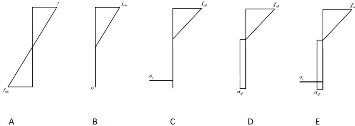
**2-2 Stresses in the cross section, A: Uncracked concrete; B:) Plain concrete; C:) Reinforced concrete; D:) Steel fibre concrete; E:) Steel fibre reinforced concrete**
