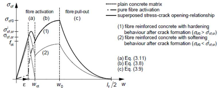
Stress – strain / crack width diagram for a ultra high strength concrete bar
