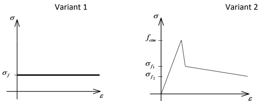
8-1 Stress strain diagram of variant the both variants
