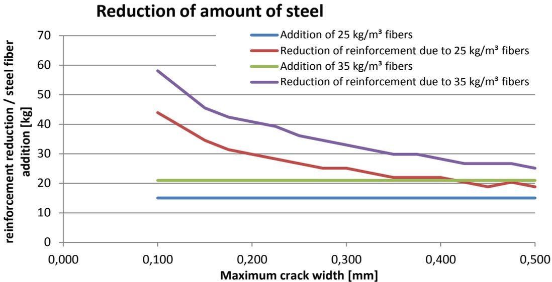
7-11 Reduction of the amount of steel in the cross section
