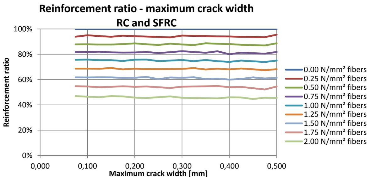
The reduction of the reinforcement, which is found in the figure before can be rewritten as a ratio of the reinforced concrete floor without steel fibres. In this figure can be seen that the amount of reinforcement can be reduced with about 55% in the case of 2.00 N/mm<sup>2</sup> fibres.
