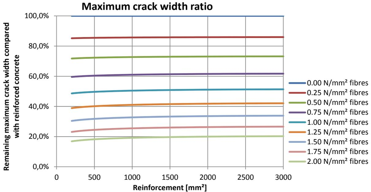
5-7 Remaining maximum crack width compared with reinforced concrete
