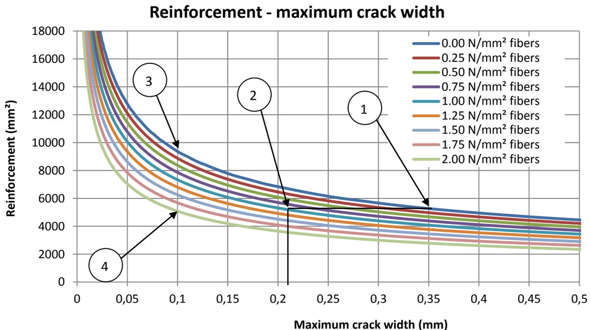
6-2 Reinforcement over maximum crack width diagram
