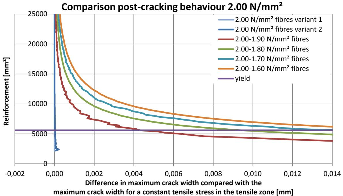
8-4 post-cracking behaviour with  $\sigma_f=2.00 \text{ N/mm}^2$
