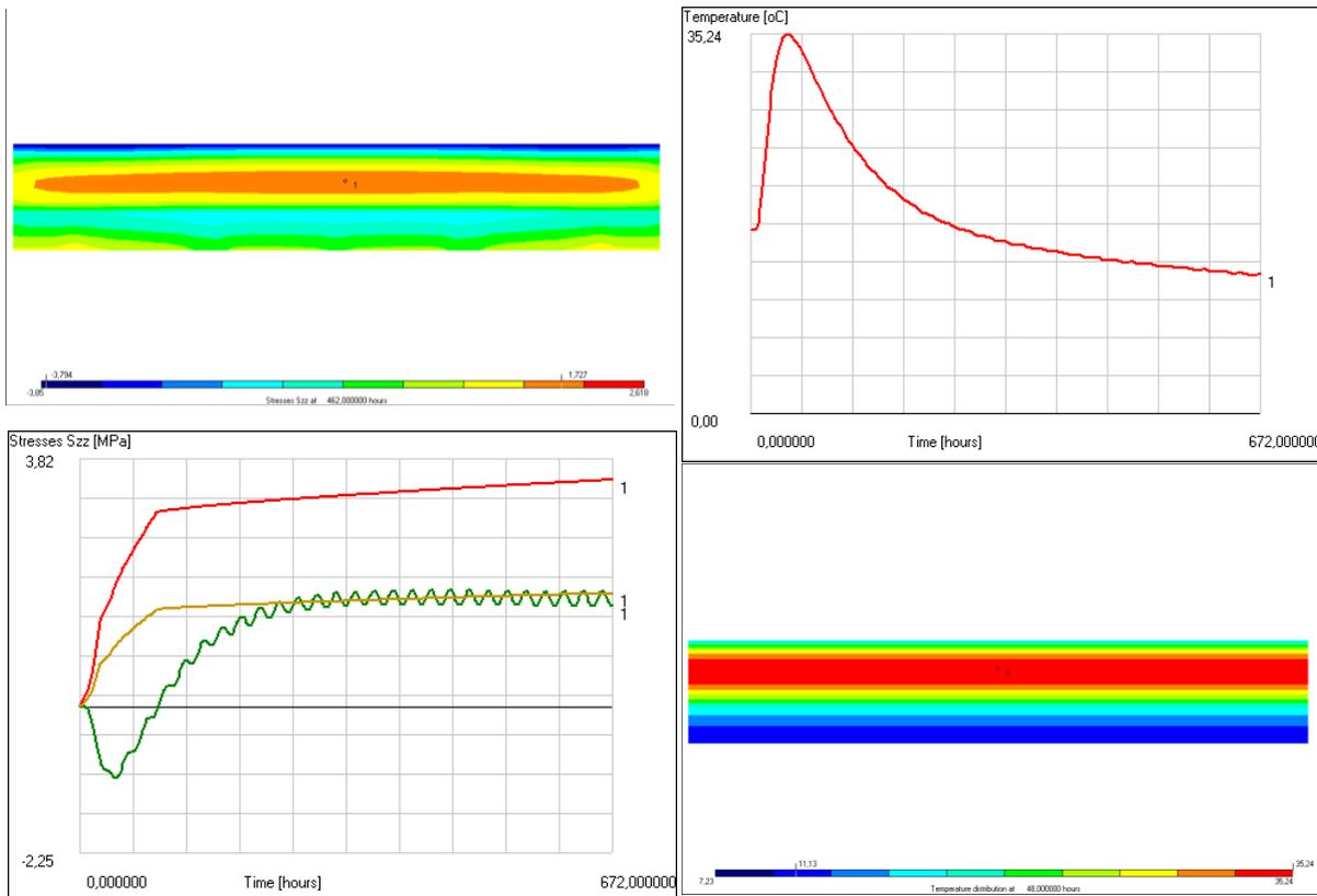
Development of the stresses due to the thermal shrinkage
