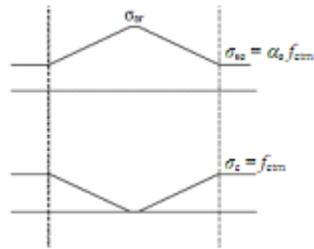
Fig. 3-4 Concrete and steel stress close to a crack in RC
