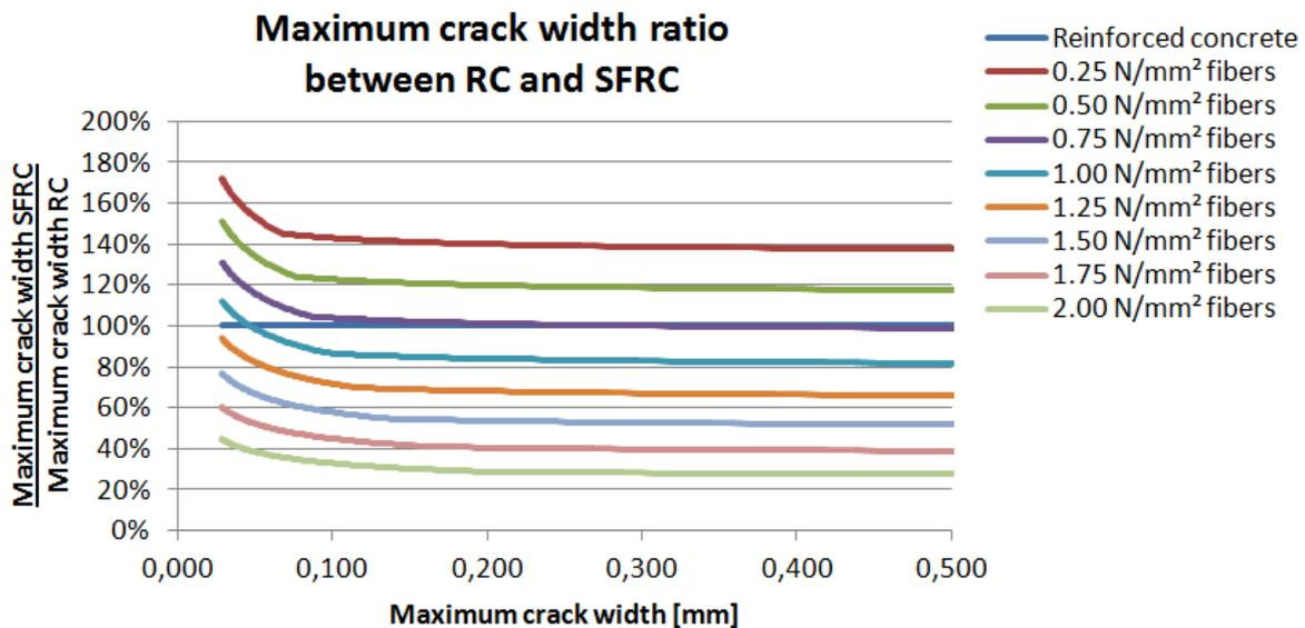
7-10 Maximum crack width SFRC compared with the maximum crack width of reinforced concrete
