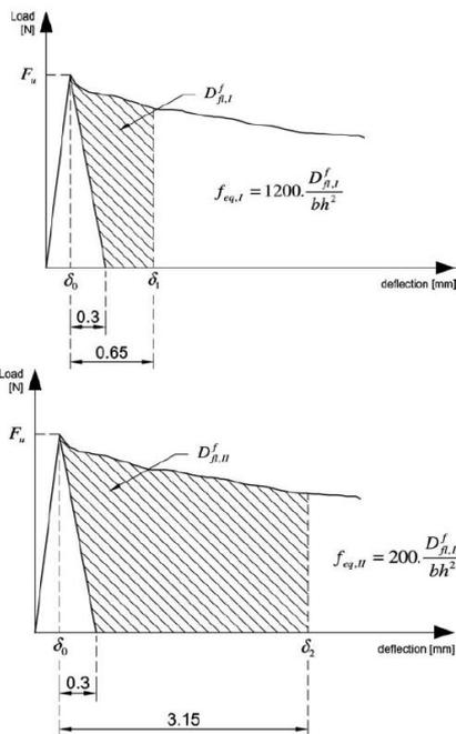
Flexural tensile stresses according the 4-points bending test
