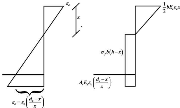
4-1 Strain and stress diagram of steel fibre concrete
