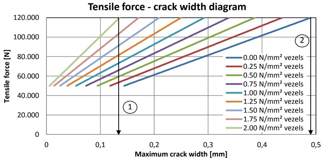
**5-2 Tensile force - crack width diagram axial tensile bar**
