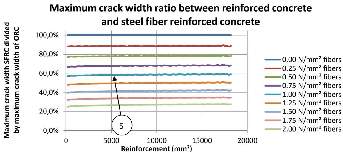
6-3 Crack width ratio between reinforced concrete and steel fibre reinforced concrete
