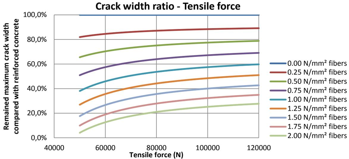
5-3 Maximum crack width ratio over tensile force
