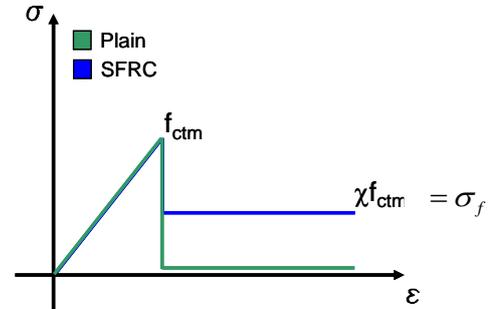
3-2 The post-cracking behavior of concrete with and without steel fibers
