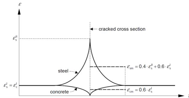
Steel and concrete strain diagram close to a crack
