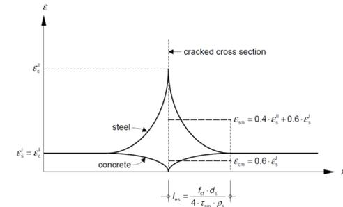
Fig. 3-6 Concrete and steel stress close to a crack in HSC
