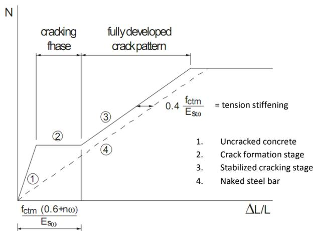
4-4 Tension stiffening model axial tensile bar
