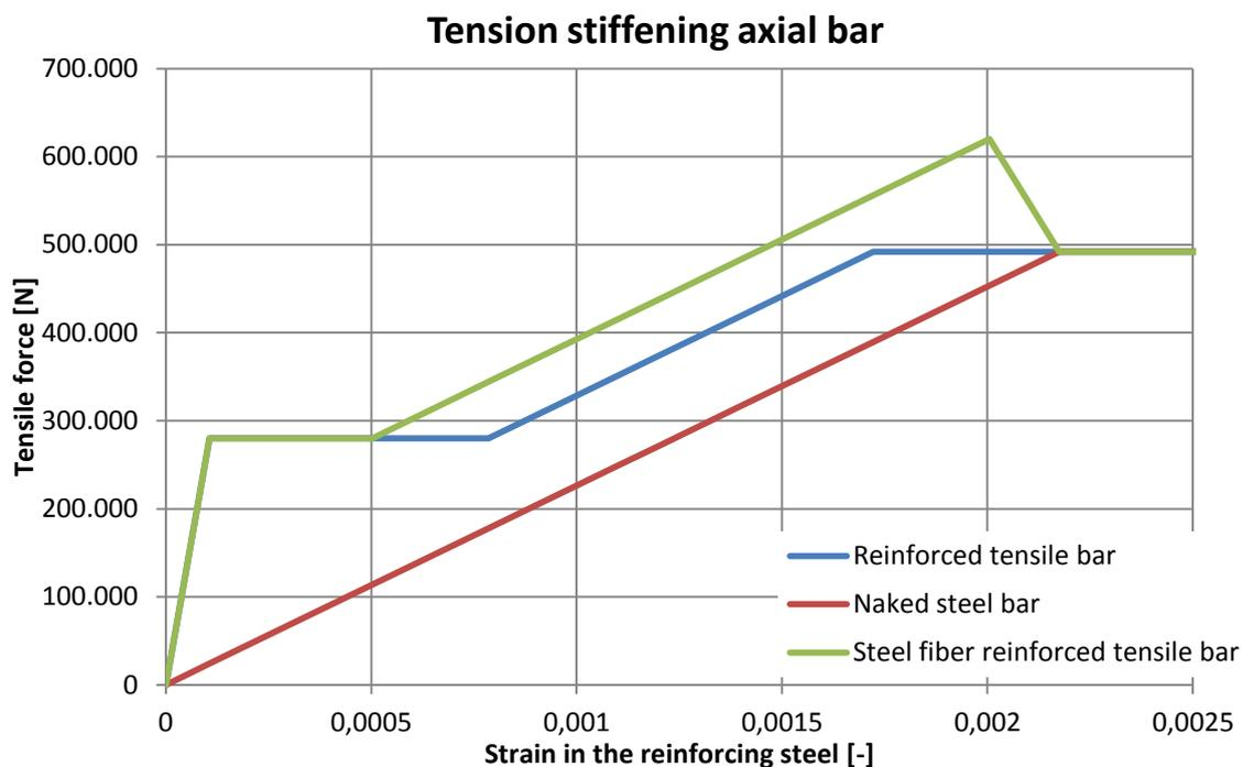
4-5 Load deformation diagram for an axially loaded tensile member with and without steel fibres
