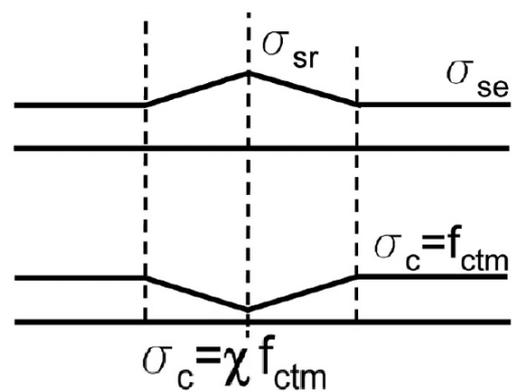
3-3 The course of reinforcing steel and concrete stresses at both sides of a crack during the transmission length
