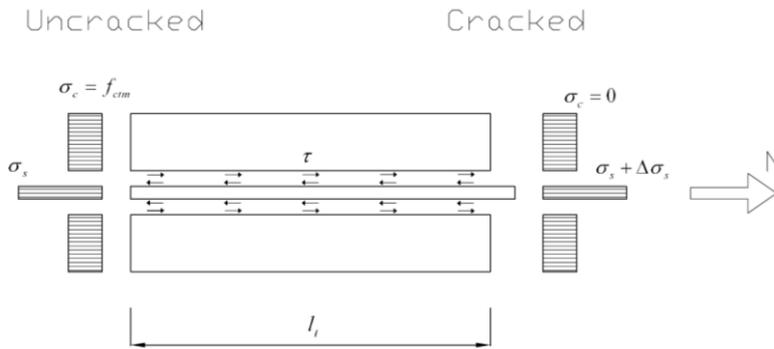
Stresses in cross section in cracked and uncracked situation
