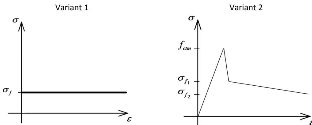
2-1 Stress-strain diagram performance-based principle
