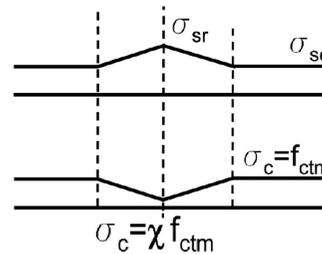
3-5 Concrete and steel stress close to a crack in SFRC
