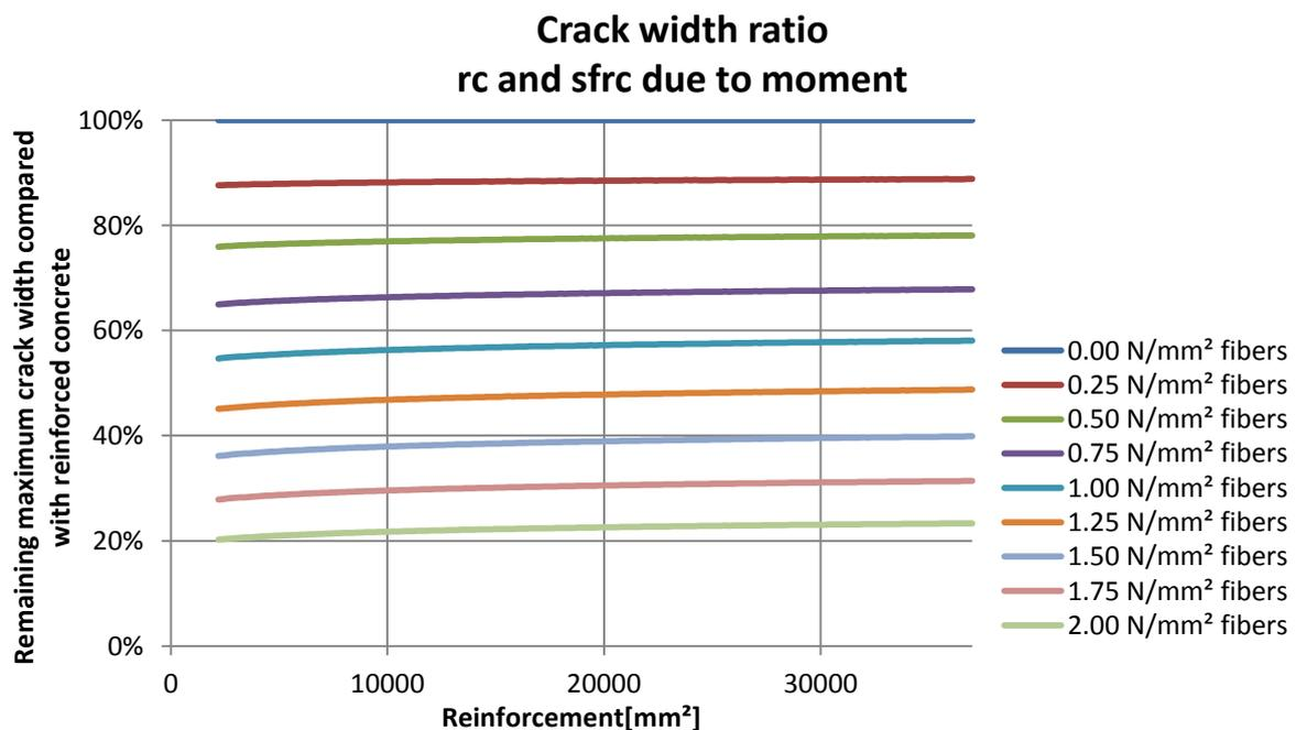
In the figure above the remaining maximum crack width is plotted if steel fibres are added. The results of the steel fibre reinforced floor are compared with the floor without steel fibres. Over the whole range of reinforcement, a near constant reduction can be seen.
