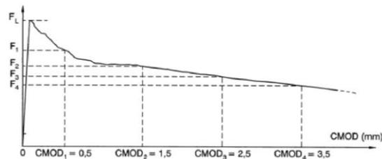
Load-CMOD diagram Rilem method
