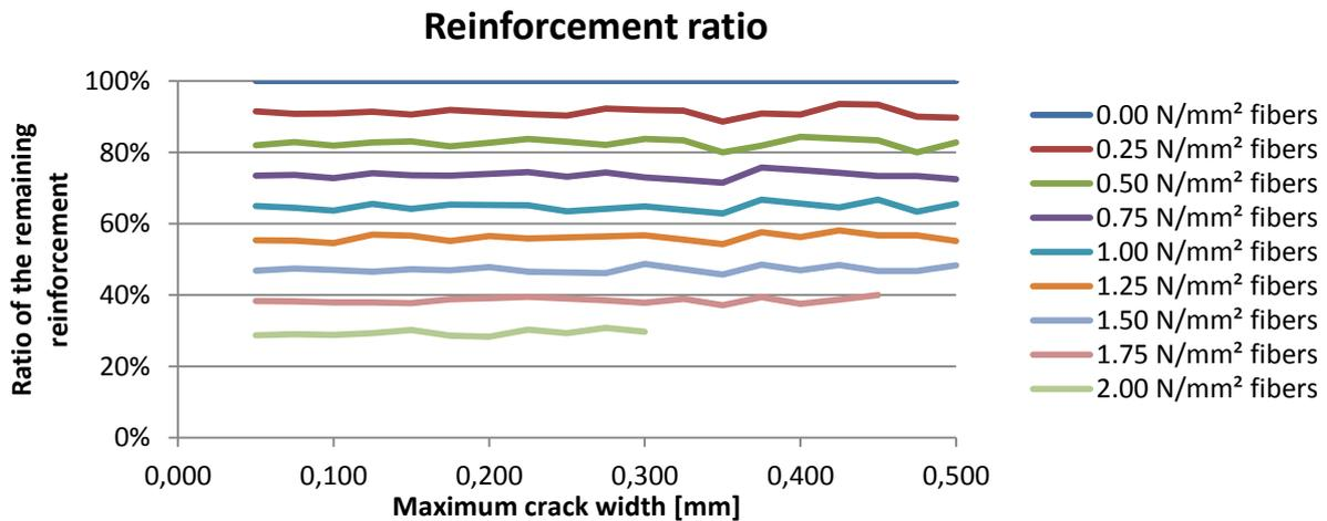
7-7 Ratio of the remaining reinforcement between RC and SFRC
