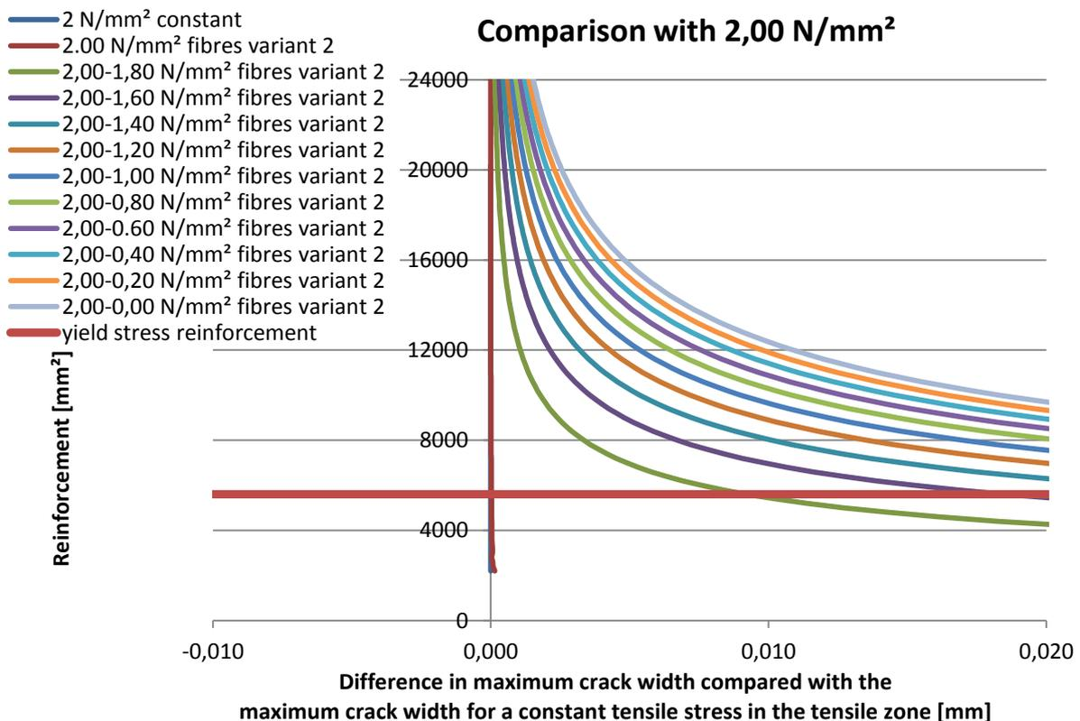
8-6 Comparison post-cracking behaviour with 2.00 N/mm<sup>2</sup>
