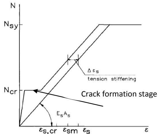
3-8 Tensile force – strain curve of a reinforced tensile member by Noakowski
