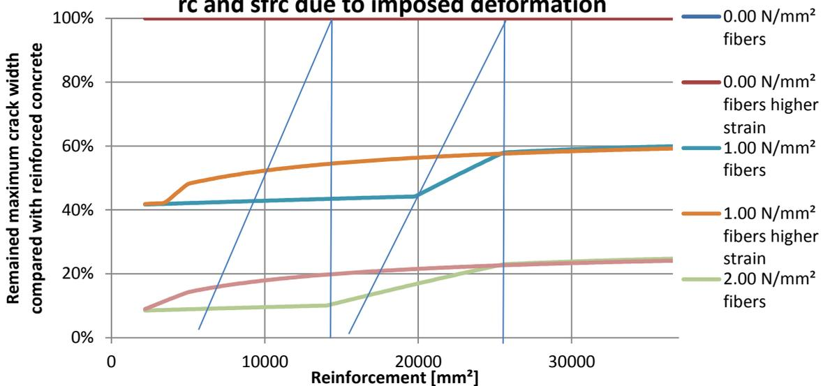
The figure above shows the remaining maximum crack width in the case of a higher strain (two times the original strain), compared with the reinforced concrete floor (for both situation the maximum
