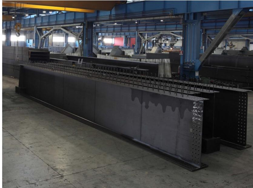
Figure 1.7: Steel plate girder
