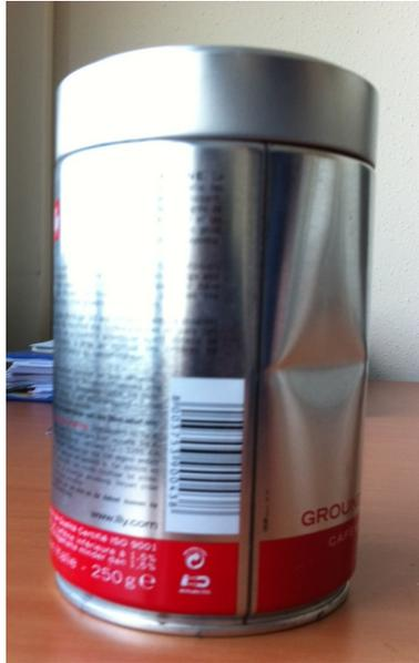
Figure 3.2: A geometric imperfection illustrated as a crease in a cylinder
