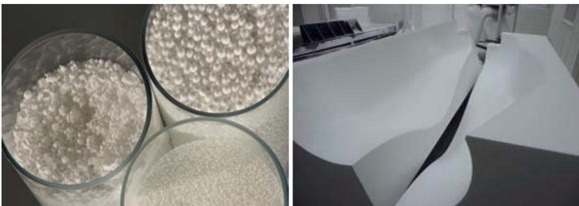
**Figure 8.3.** Left: unprocessed EPS; Right: EPS concrete mould created by 3D-milling (Wapperom,2004)
