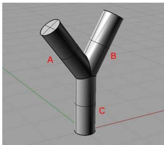
**Figure 3.17.** Structural node in UHPC
