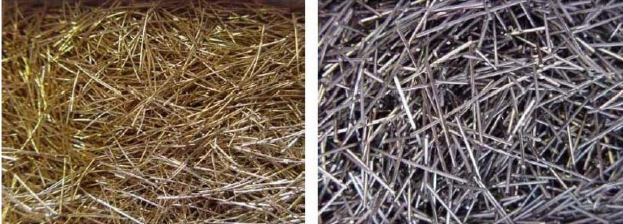
**Figure 2.5.** Left, high strength steel fibres  $L/D = 6/0,15$  mm; right, steel fibres  $L/D = 12,5/0,4$  mm (www.bekaert.com).
