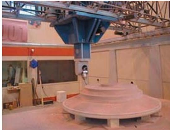
**Figure 8.4.** Five-axis milling-machine ([www.nedcam.nl](http://www.nedcam.nl)).
