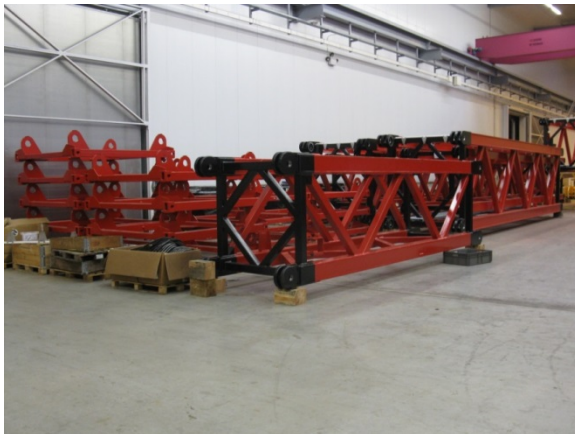
Figure 2-3: Disassembled parts which can be transported on containers
