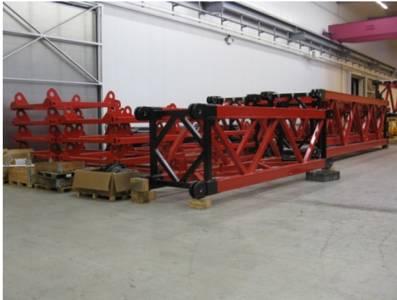
Figure A-8: Disassembled parts which can be transported on containers
