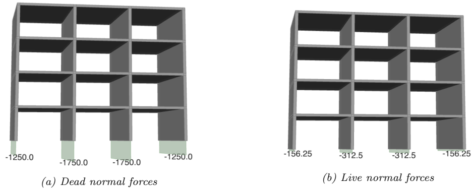
Figure 6.17: Tool normal forces
