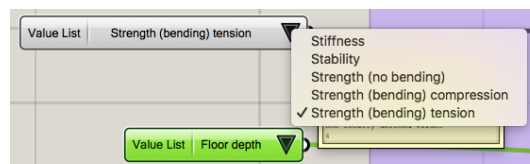
Figure 6.12: Feasibility checks offered by the tool, visualised in Rhino-Grasshopper
