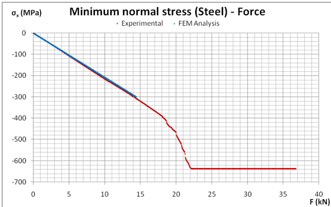
Figure 6.12 Normal stresses – force diagram for the steel plate of specimen BSC4
