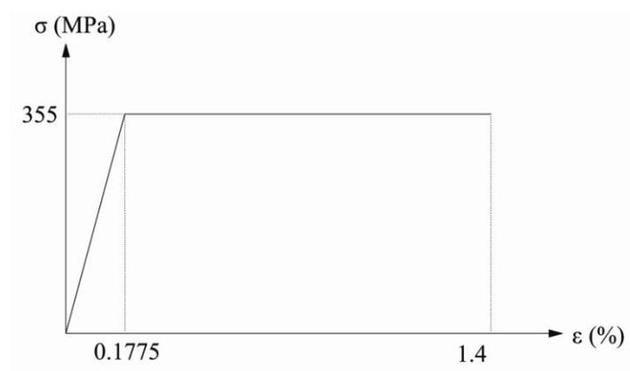
Figure 6.2 Bilinear stress – strain diagram for steel
