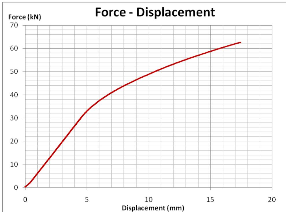
*Figure 4.51 Force against vertical displacement diagram for specimen BSC3*
