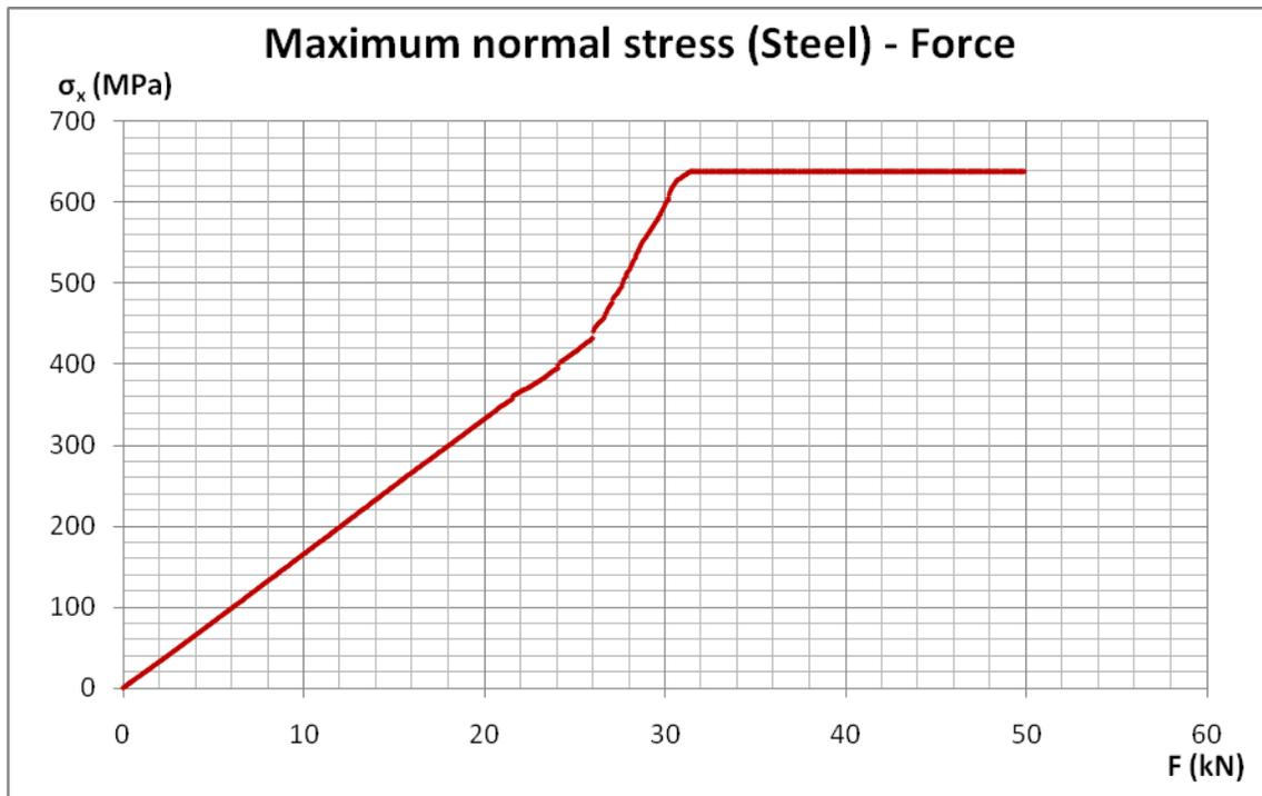
Figure 4.65 Maximum normal stress (located at the outer surface of the steel plate) against force diagram of specimen BST1
