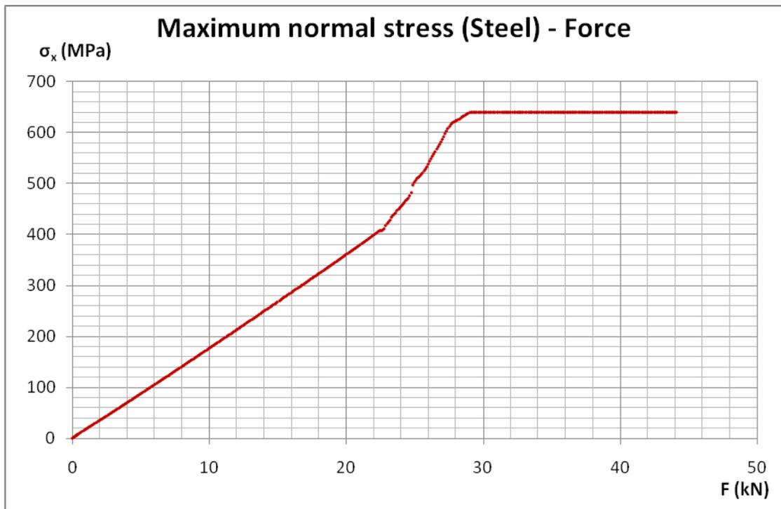
Figure 4.71 Maximum normal stress (located at the outer surface of the steel plate) against force diagram of specimen BST2
