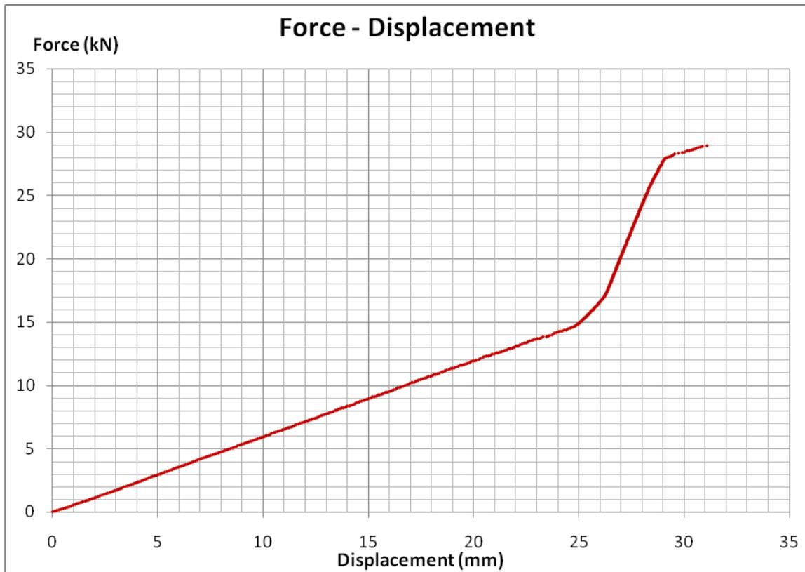
*Figure 4.29 Force against vertical displacement diagram for BP4*
