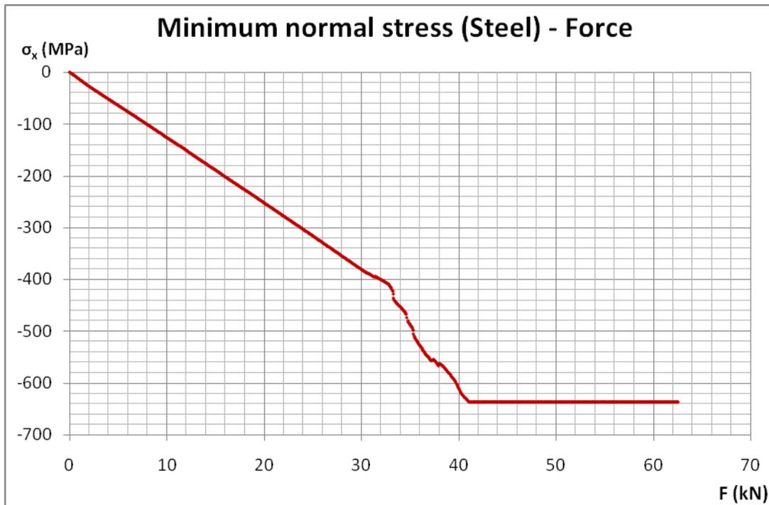
Figure 4.52 Minimum normal stress (located at the outer surface of the steel plate) against force diagram for specimen BSC3
