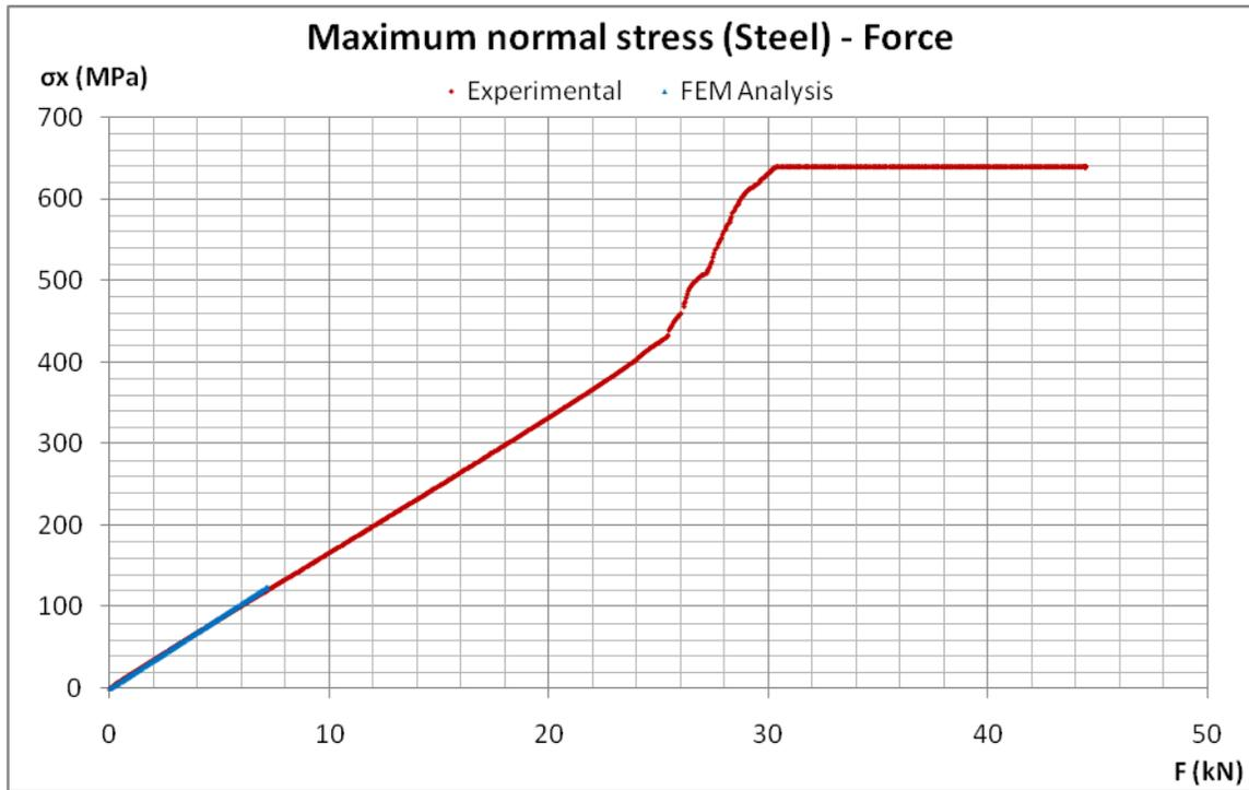
Figure 6.24 Normal stresses – force diagram for the steel plate of specimen BST3
