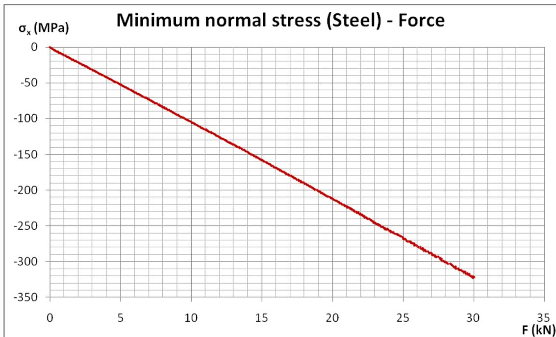
Figure 4.46 Minimum normal stress (located at the outer surface of the steel plate) against force diagram for specimen BSC2
