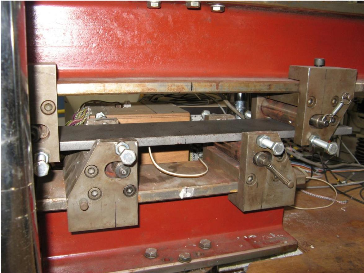
*Figure 4.87 Experimental configuration for the steel plate*
