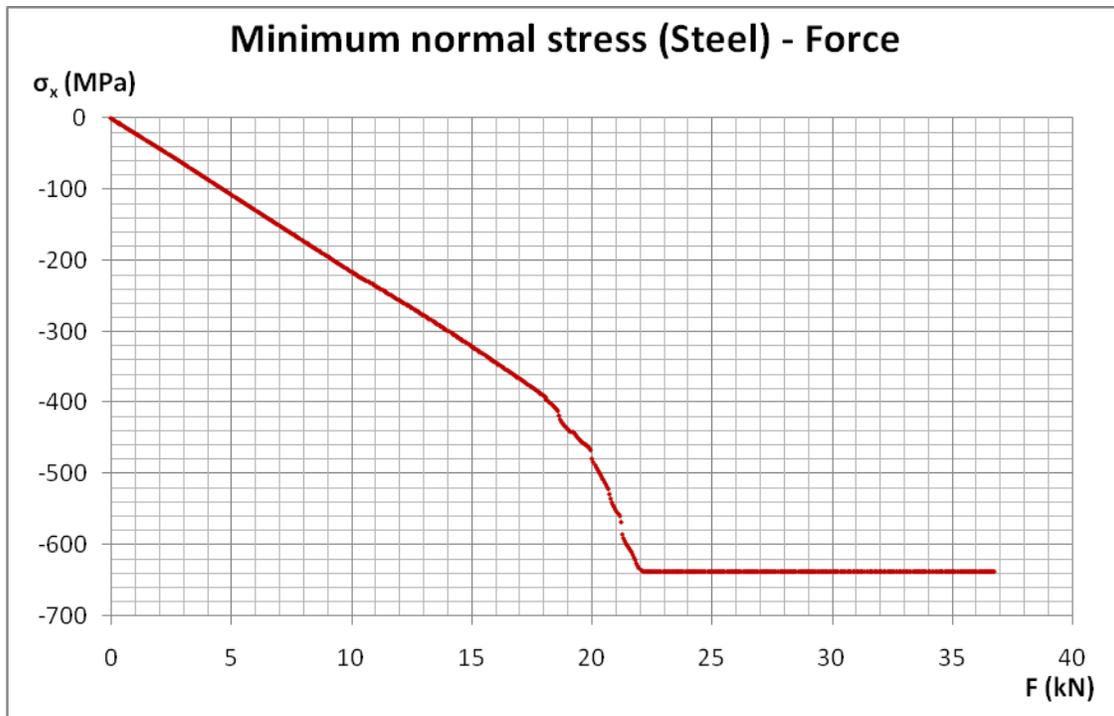
Figure 4.58 Maximum normal stress (located at the outer surface of the GFRP plate) against force diagram for specimen BSC4
