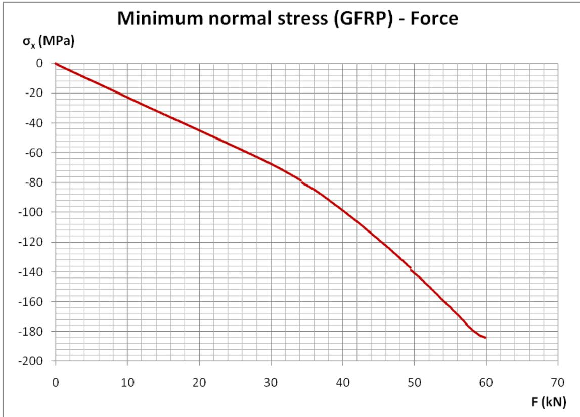
*Figure 4.78 Minimum normal stress (located at the outer surface of the GFRP plate) against force diagram for specimen BST3*
