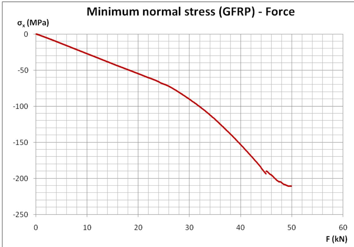
*Figure 4.66 Minimum normal stress (located at the outer surface of the GFRP plate) against force diagram for specimen BST1*
