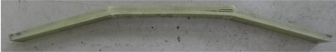
*Figure 4.22 Failed GFRP specimen BP4 in bending*
