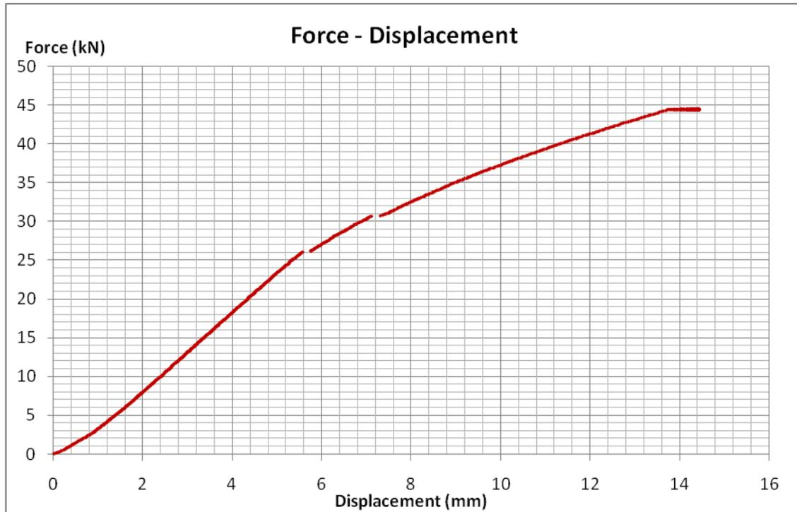
Figure 4.82 Force against vertical displacement diagram of specimen BST4
