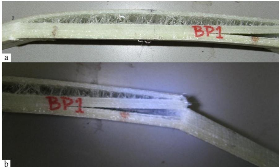
*Figure 4.18 Details of failed GFRP specimen BP1 in bending*
