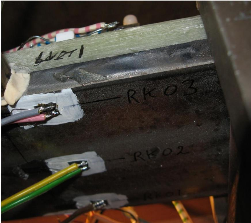
*Figure 4.34 Strain gauges on the steel plate in the mid span area*
