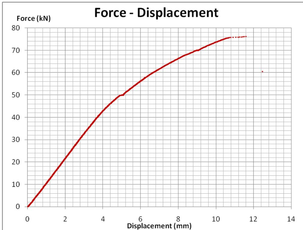
*Figure 4.39 Force against vertical displacement diagram for specimen BSC1*
