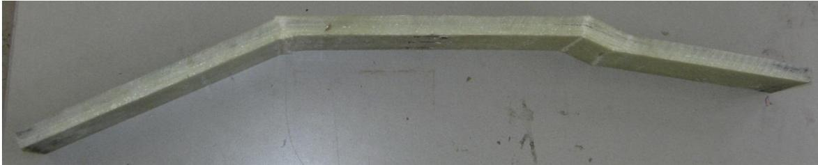
*Figure 4.20 Failed GFRP specimen BP3 in bending*
