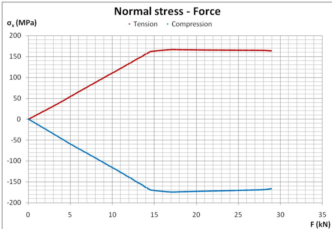
Figure 4.30 Maximum and minimum stress against force for specimen BP4
