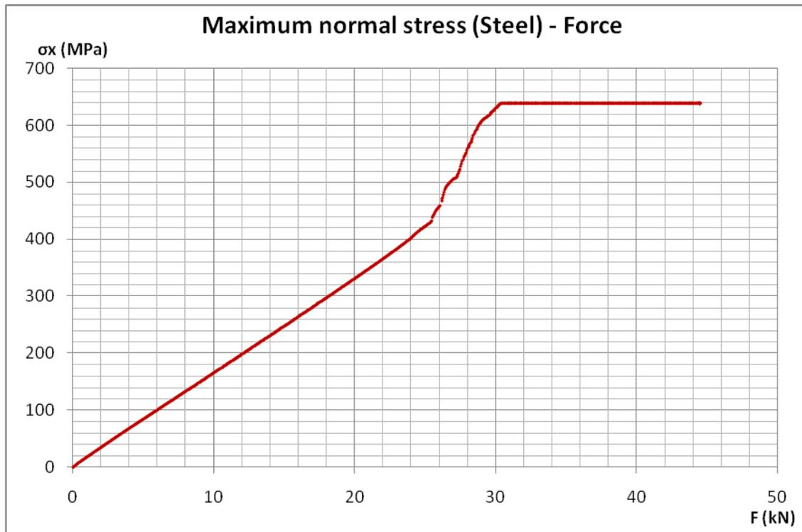
Figure 4.83 Maximum normal stress (located at the outer surface of the steel plate) against force diagram of specimen BST4
