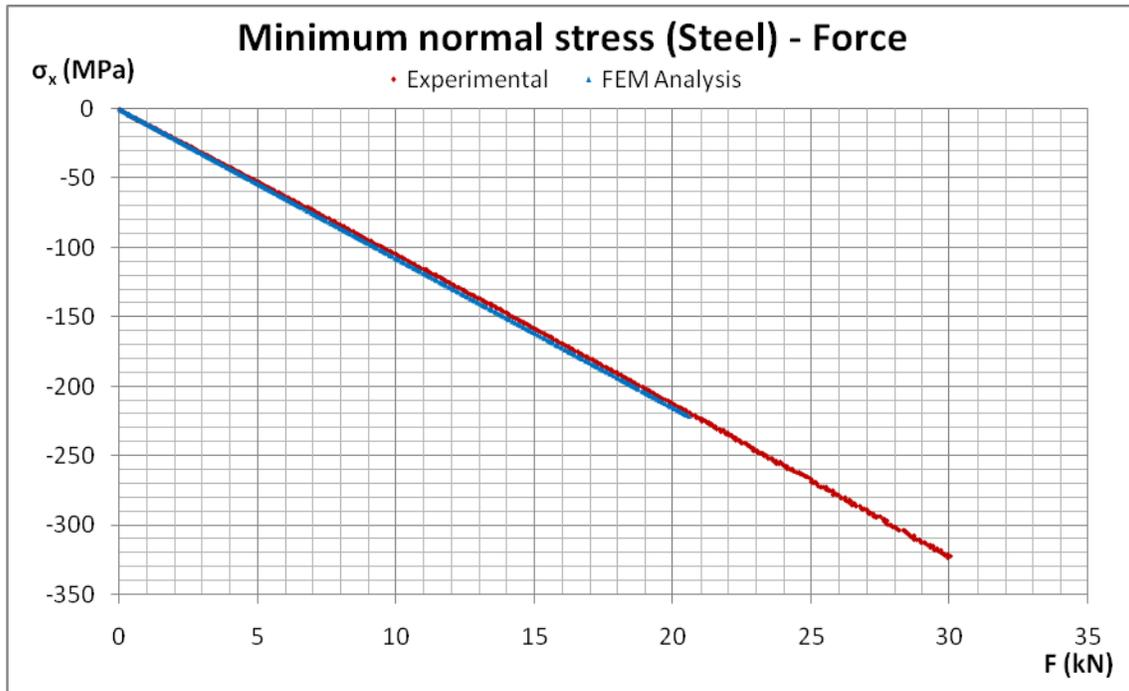
*Figure 6.4 Normal stresses – force diagram for the steel plate of specimen BSC2*
