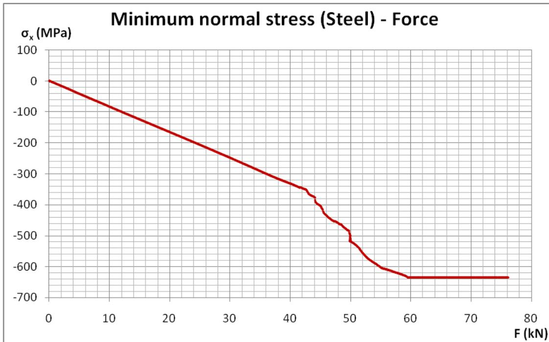
Figure 4.40 Minimum normal stress (located at the outer surface of the steel plate) against force diagram for specimen BSC1
