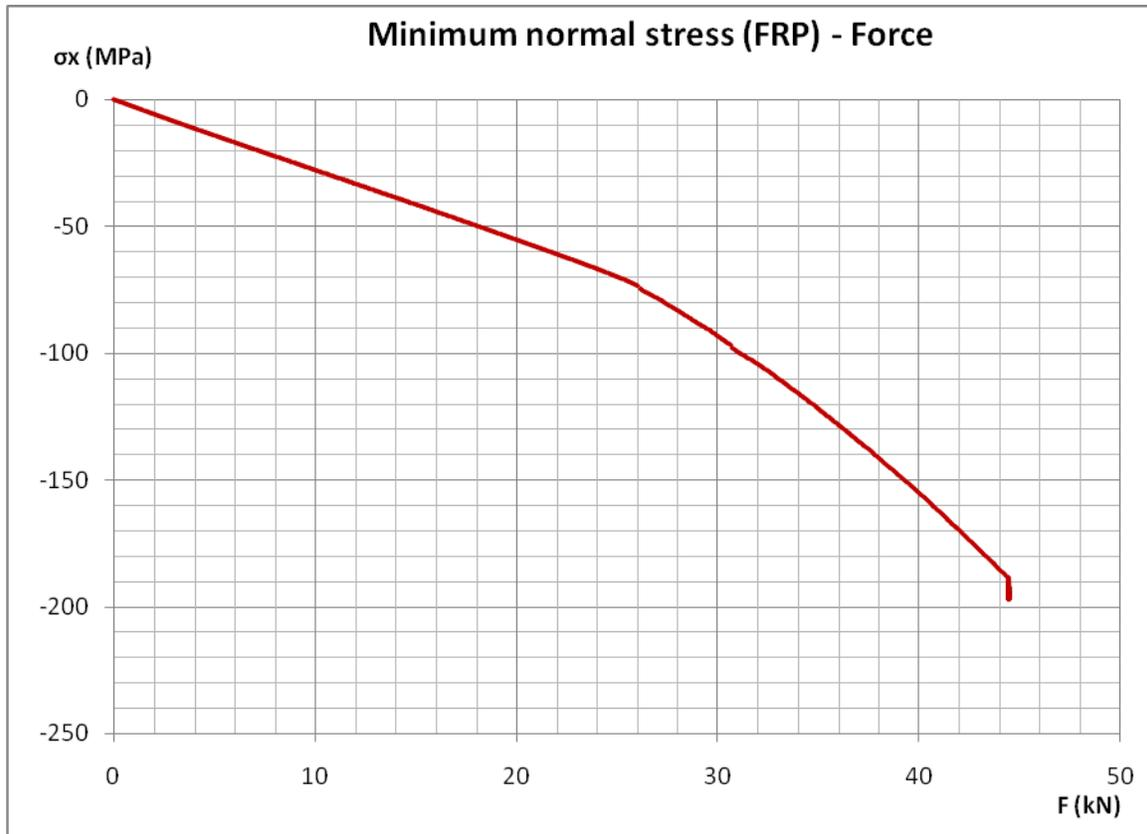
*Figure 4.84 Minimum normal stress (located at the outer surface of the GFRP plate) against force diagram for specimen BST4*
