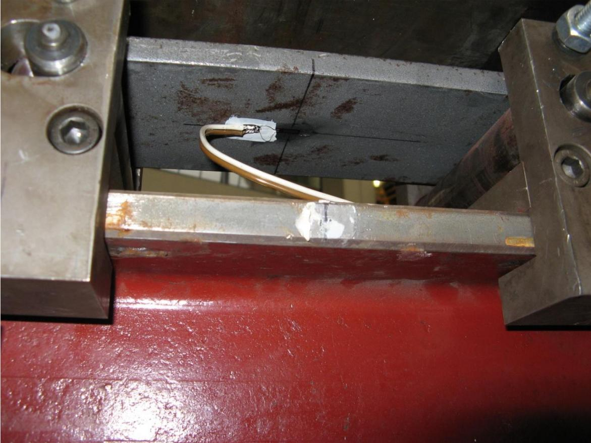
*Figure 4.88 The strain gauge at the mid span area on the steel plate*
