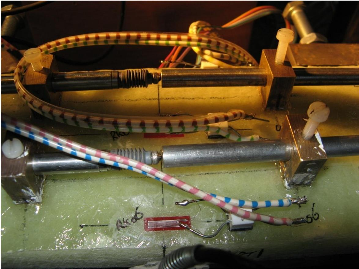
*Figure 4.93 Strain gauges on the FRP plate in the mid span area*
