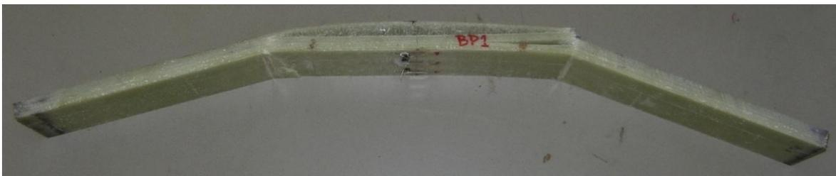
*Figure 4.17 Failed GFRP specimen BP1 in bending*
