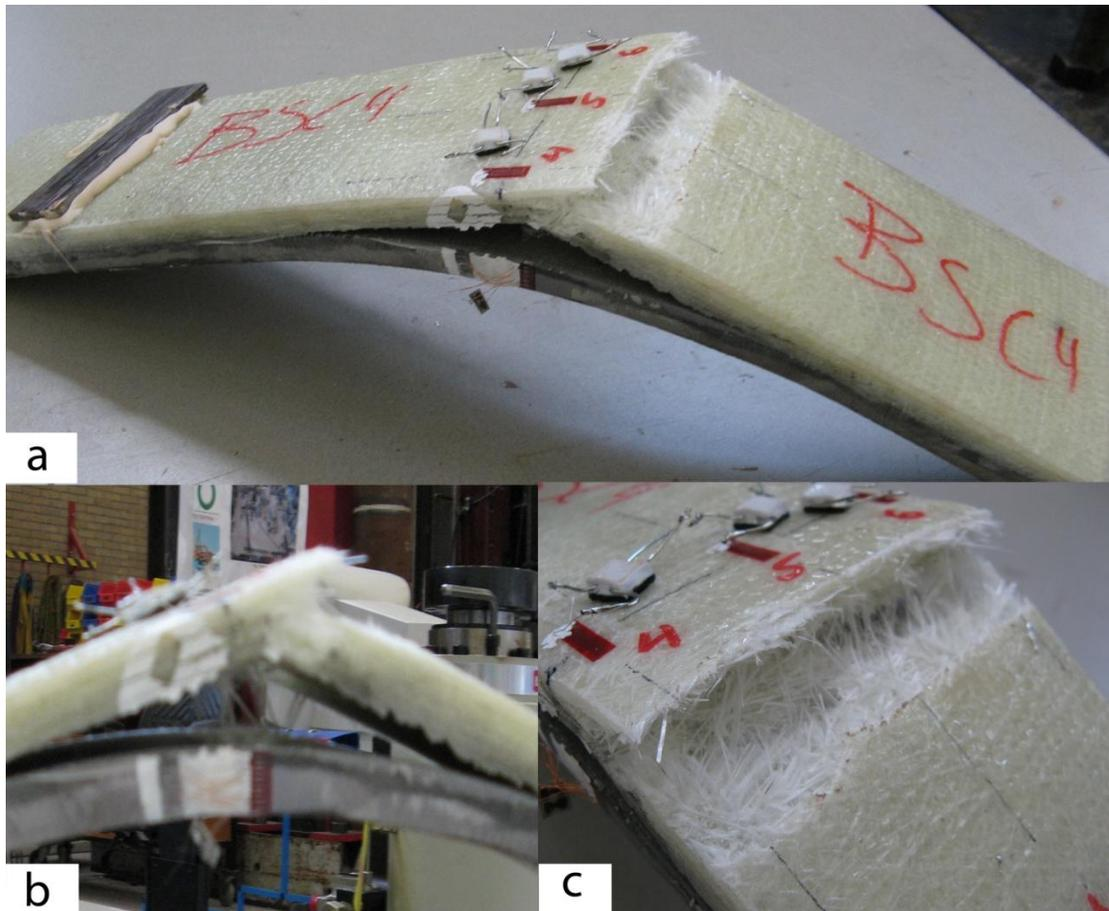
*Figure 4.56 Failure and details of specimen BSC4*
