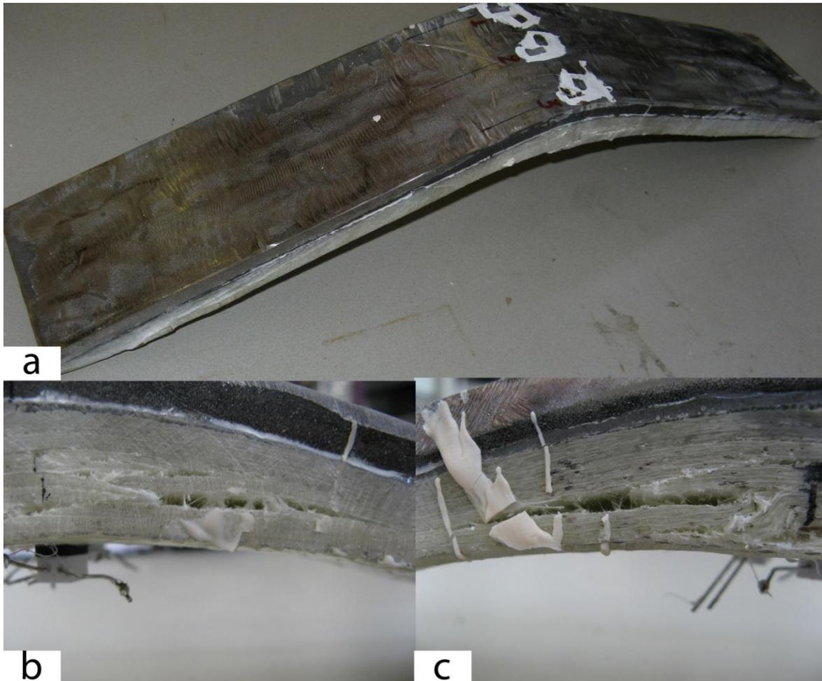
*Figure 4.63 Failure and details of specimen BST1*
