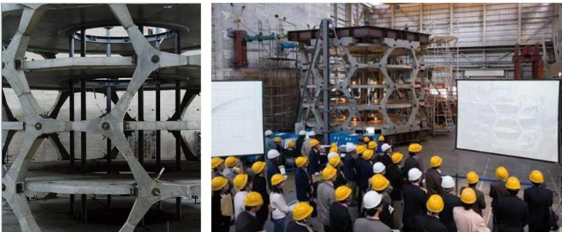
Fig.5.9 full scale model and test (The resulted capacity is 6 times of self-weight)
