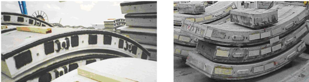
**Figure 2.4:** Tunnel segments with kaubit used as a packing material (left) and plywood used as a packing material (right)
