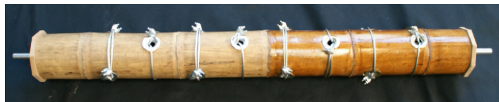
Figure 2.9: Multi-knot lashing joint (Widyowijatnoko, 2012)
