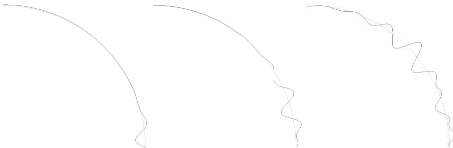
Figure 13.6. Buckling modes 1, 3 and 6 for a hinged supported axisymmetrical shell subjected to vertical load
