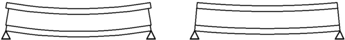
Figure 118: Deck structure as modeled in original tender design (left), Real behavior of deck structure (right)
