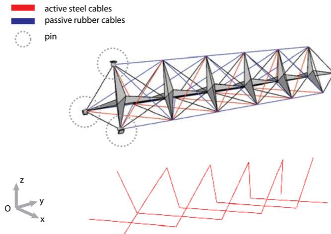
Image 2.89. Assembly actuators and constrains.
