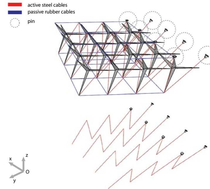
Image 2.93. Assembly actuators and constrains.
