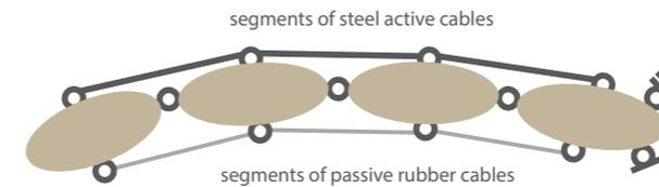
Image 4.19. Segments of steel active cables control the motion.
