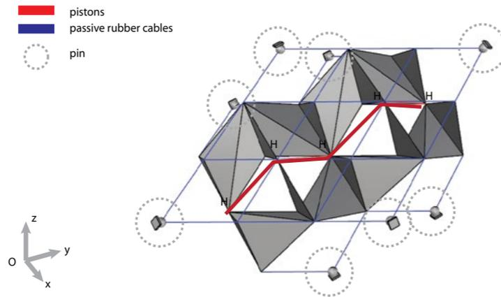
Image 2.78. Assembly actuators and constrains.
