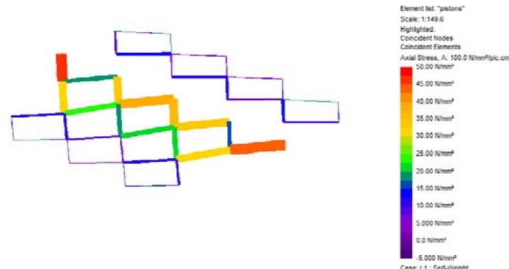
Configuration #2. Max tensile stress 48.2 MPa. Max compressive stress 13.1 MPa Load Case A1.
