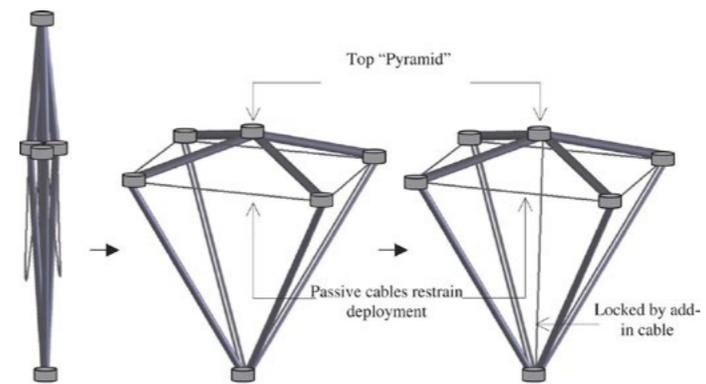
Image 2.70. A by-pyramid simplex (image courtesy of Vu et al 2003).
