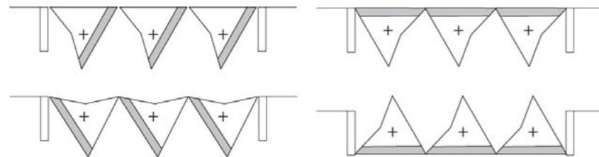
Image 3.22. Possible arrangements in section of the rotatable prisms used on the walls and ceiling (Top left) specularly reflective; (Bottom left) scattering; (Top right) absorbing; and (Bottom right) highly scattering (image courtesy of Barron 2009).
