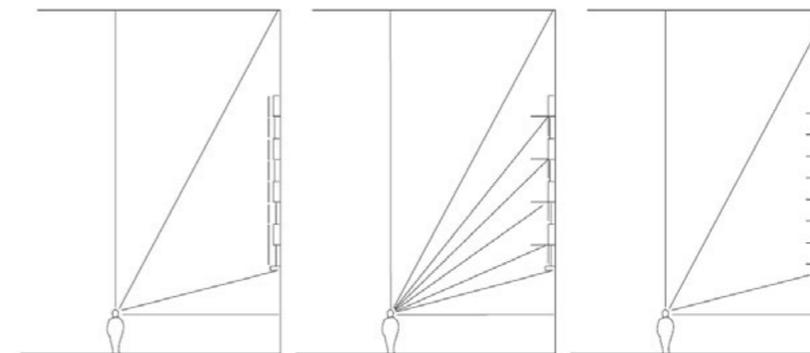
Image 3.18. Variable absorption in the Hong Kong Academy for Performing Arts. The three arrangements of flaps allow three degrees of absorptive panles to be exposed, (Left) Flaps – all closed for long reverberation time; (Center) flaps – half open for medium reverberation time; (Right) flaps – all open for short reverberation time (image courtesy of Barron 2009).
