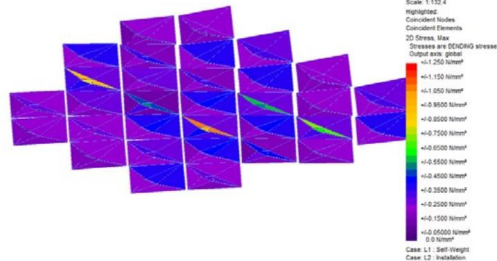
Configuration #3. Max stress 0.98 MPa. Load Case A1.
