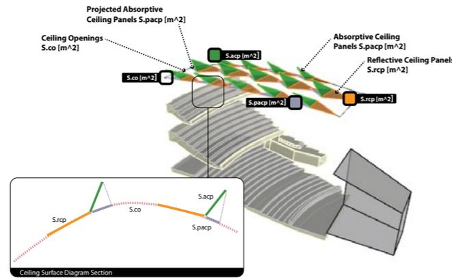
Image 3.29. Modelling of a sampling variable acoustic ceiling: in orange the reflective panels, in green the absorptive ones, and in lavande the effective absorptive panel area as projection on the ceiling surface definition.
