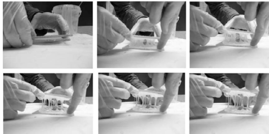
Image 2.60. Form-finding process with a viscous material (image courtesy of Andrés Harris).
