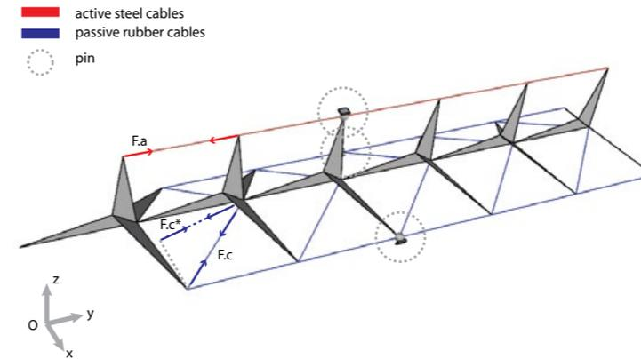
Image 2.88. Assembly actuators and constraints.
