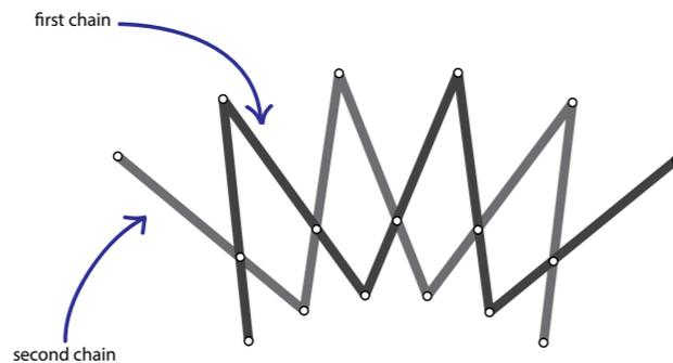
Image 2.20. Two interwoven kinematic chains form a curved linear SLE deployable element.
