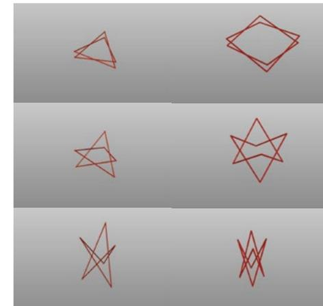
Image 2.21. Deployment process of a trissor and a tetrascissor element.
