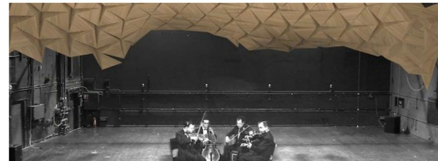
Image 4.06. An architectural rendering for an extense solution of the Resonant Chamber prototype. When the surface deploys, extra absorbing area is provided.
