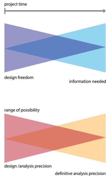
Image 3.25. Top: design freedom vs. amount of information (image courtesy of ir. J.L. Coenders; in turn adapted from MacLeamy curve). Bottom: envisioned use of different precision-defined tools for the assessment along design time.
