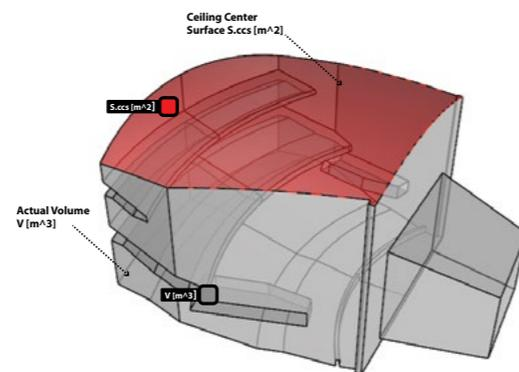
Image 3.27. Effective volume of the hall after being trimmed by the ceiling surface definition.
