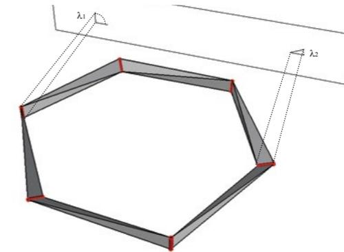
Image 2.33. Parameters for revolute joint typologies.
