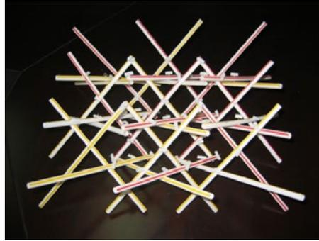
Image 2.26. Expandable arch based on a grid of Bennett linkages (image courtesy of Zhong You).
