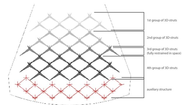
Image 4.16. Groups of structural elements composing the kinetic system and auxiliary substructure.
