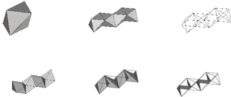
Image 2.77. Generation of structure starting from an octahedron.
