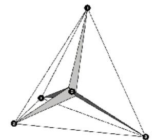
Image 2.81. A 3D-rigid body generated from a tetrahedron.
