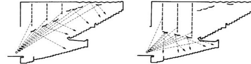
Image 4.05. The Cain Auditorium has a vertically movable ceiling system (Image courtesy of Ballou et al 1987)
