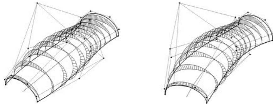
Image 1.8. Parametric model of a roof with efficiently shaped trusses (image courtesy of Lorenz Lachauer, ETHZ).
