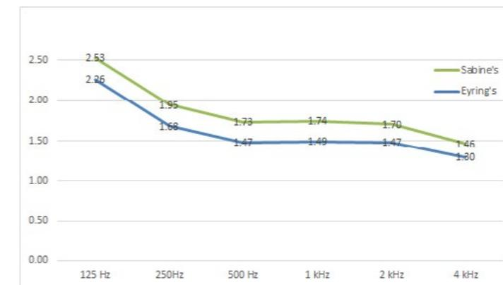
Graph 5.01. Reverberation Time (sec) versus sound frequency (kHz) for the first configuration.
