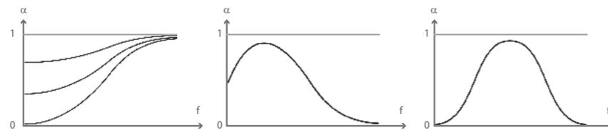
Image 3.13. Typical Absorptive spectrum for (starting from the left) a porous, a vibrating membrane and Helmholtz resonator.
