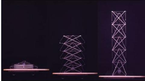
Image 2.7. Pantographic deployable mast (image courtesy of Z. You and S. Pellegrino).
