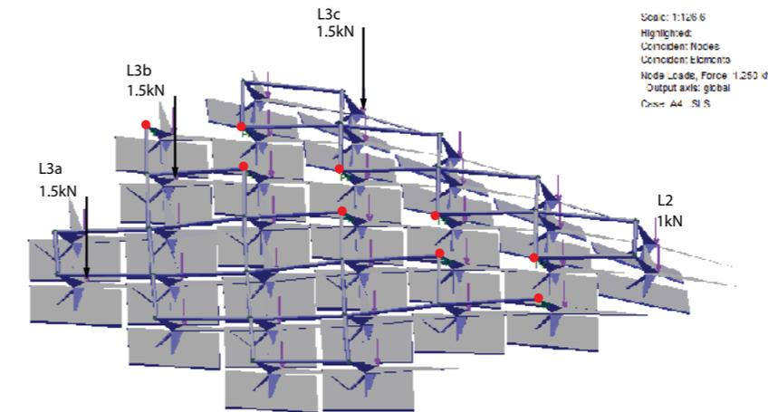
Image 5.02. Loads for the structure: in black the maintenance node loads, in three different locations, while in violet the installation loads.
