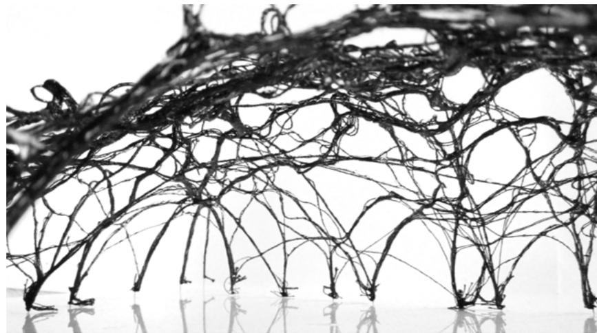
Image 2.8. Form-finding physical model based on Frei Otto's studies about form emergence and optimal minimum path (image courtesy of WeWantToLearn.net).
