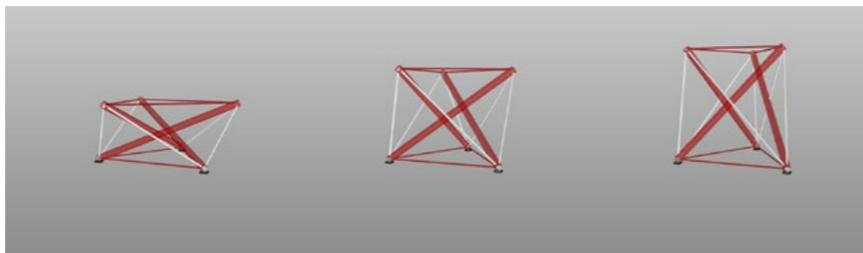
Image 2.73. Motion of an order-three tensegrity prism while releasing the three active cables.
