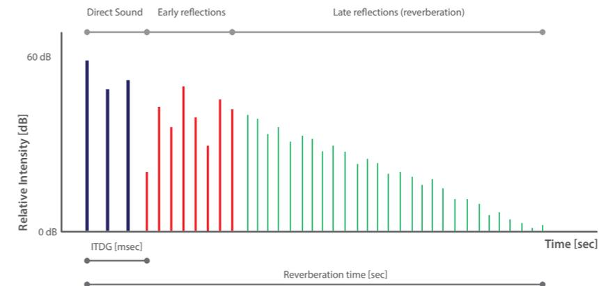
Image 3.5. Reflectogram showing direct sound (in blue), early reflections (in red) and reverberation (in green).
