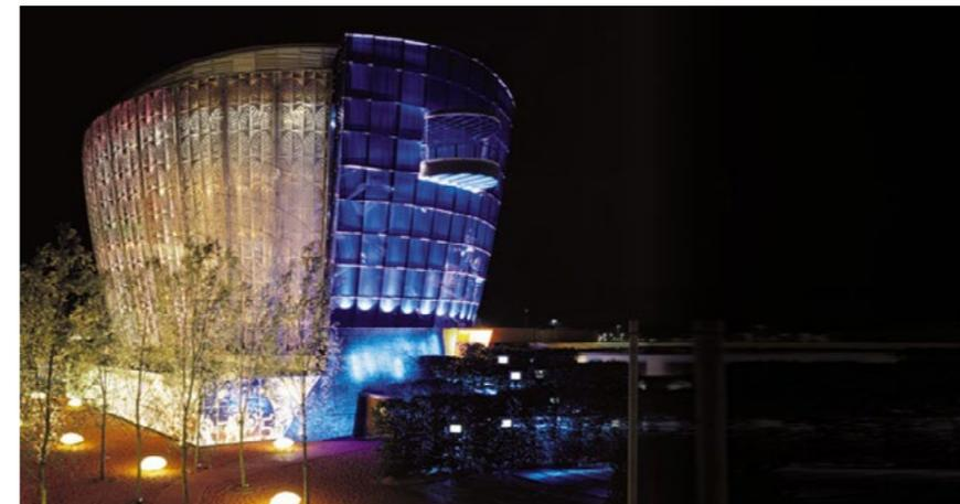
Image 2.1. An example of dynamic structure (Lelieveld 2013): Cyclebowl, Atelier Brückner design. Pneumatic control of roof and façade transparency. Sensor controlled louver system.
