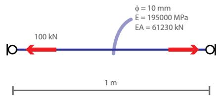
Image 2.64. A prestressed cable pinned at its ends
