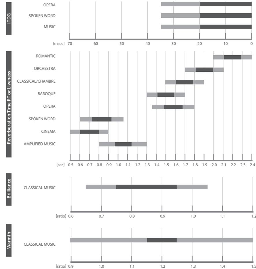
Table 3.3. measurement range of acoustic criteria and performance type: in dark grey the optimal and in light grey the acceptable ones.
