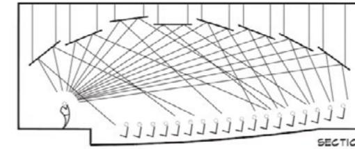
Image 4.27. A ceiling system having different surface curvature according to directional needs. (image courtesy of Long 2006)
