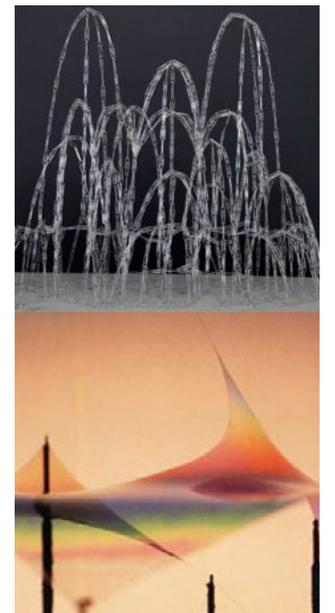
Image 2.62. Top: Church of Colònia Güell model, Antoni Gaudí desing. Bottom: Soap film model for a membrane structure (image courtesy of ILEK).
