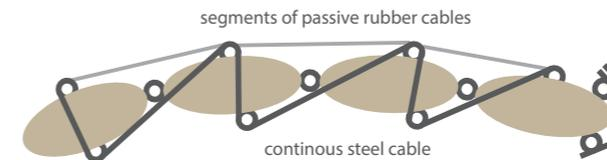
Image 4.20. A continuous steel active cable controls the motion.
