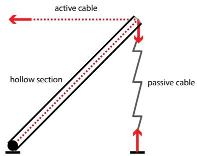
Image 2.72. Basic Mechanism with one strut, one active and one passive cable.
