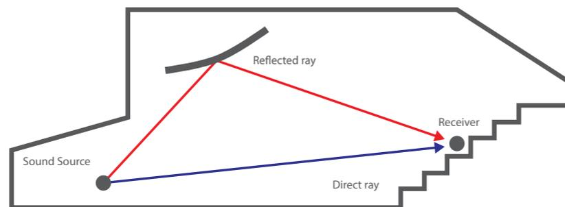
Image 3.14. Geometry for the determination of the ITDG.
