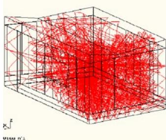
Image 3.4. Digital simulation of a diffuse sound field with 200 rays reflected in a closed room (image courtesy of Cammarata 2006).
