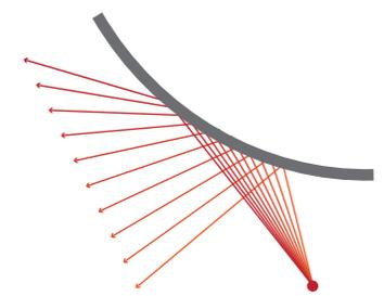
Image 4.08. A convex and a concave surface have a different interactions with acoustic rays
