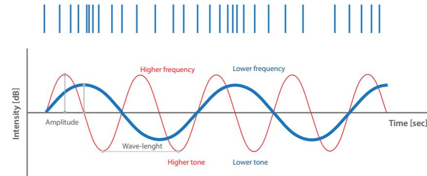
Image 3.3. Comparison of sound wavelength for two sine waves with different frequency.
