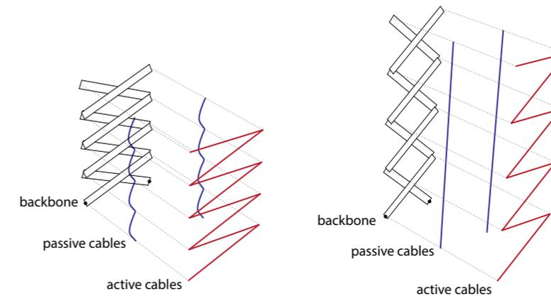
Image 2.74. Structural components for a pantographic mast (in turn adapted from Gantes 2000).
