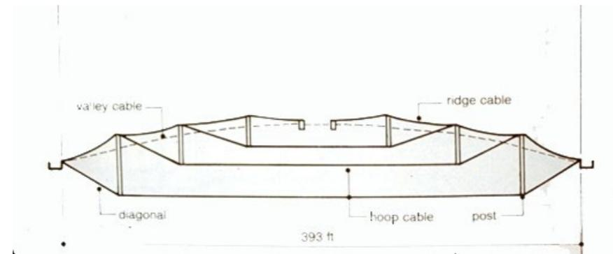
Image 2.58. Geiger's dome, an example of tension structure.
