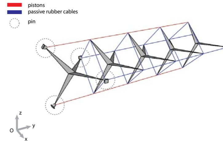
The mast can be particularly useful when a very compact configuration is needed for transportation, for instance, and then deployed. For this reason, conceptual design of this have can be envisioned for deployable mast for space application.
