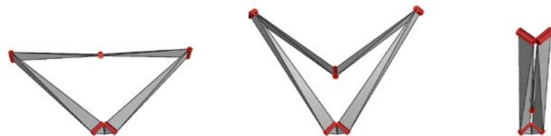
Image 2.37. Myard linkage during the folding process.
