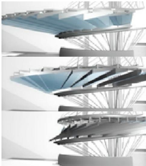
Image 2.19. Transformable Canopy SHoP and Hoberman design. The canopy is developed from a unique spiral geometry, constructed of structural panels and supported by a series of tension rods.
