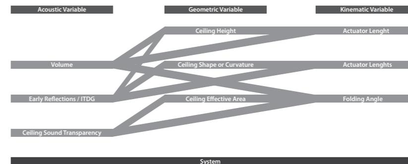
Image 4.28. An applied framework for the integrate design of the acoustic ceiling.
