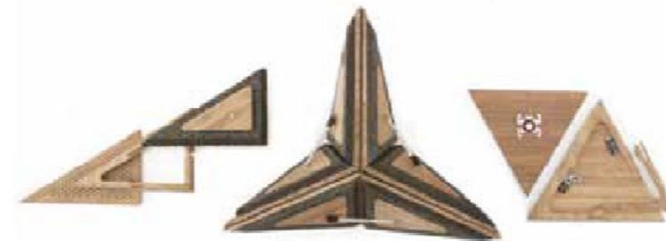
Throughout acoustic simulations, the research demonstrated that the rigid origami surface with variable absorptive and reflective panels could be configured to achieve a wide range of reverberation times, thereby offering opportunities for multiple program uses within a space (Thün 2012).
