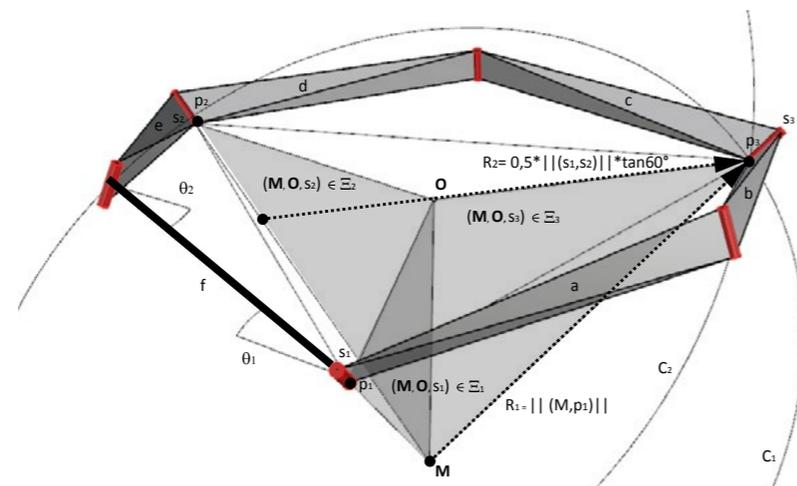
Image 2.32. Synthesis of Bricard linkage.
