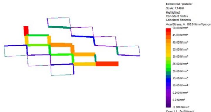
Configuration #3. Max tensile stress 46.7 MPa. Max compressive stress 9.3 MPa Load Case A1.
