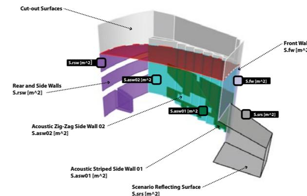
Image 3.28. Families of surface in the hall: in violet the absorptive rear and side walls, in cyan, the reflective wall, in lavande the reflective front wall and in green a further reflective tilted wall.
