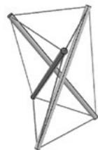
Image 2.65. Form-finding process of a tensegrity prism.
