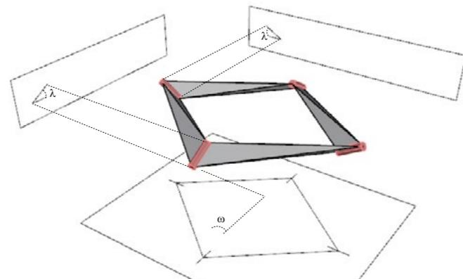
Image 2.29. Parameters for revolute joints and links.
