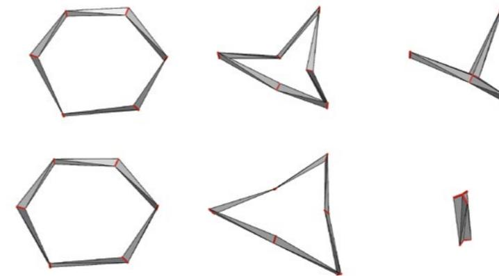
Image 2.34. Top: a partially foldable Bricard linkage with  $\lambda_1 = 90^\circ$  and  $\lambda_2 = 30^\circ$ . Bottom: a fully foldable Bricard linkage with  $\lambda_1 = 90^\circ$  and  $\lambda_2 = 60^\circ$ .
