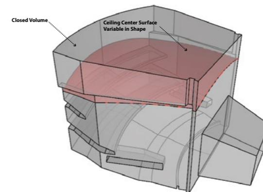
Image 3.26. Geometric 3D model of the case study, Nieuwe Luxor in Rotterdam, Bolles + Wilson architects design. 3D modelling Matteo Soru, in turn augmented from the model of Kjell Scholts. The hall has been modelled as a water-sealed volume.
