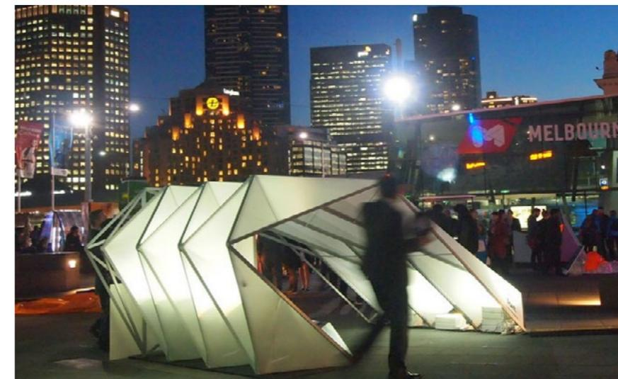
Image 2.41. EN-FOLD, Woods&Bagot design: a foldable 2D-rigid structure working as envelope (image courtesy of Woods&Bagot).
