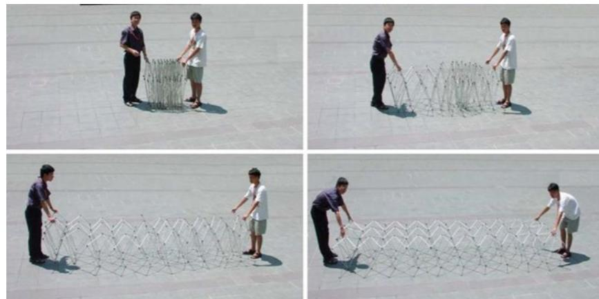
Image 2.66. A space assembly of simplex connected with passive steel cables, slacken during deployment (image courtesy Vu et al 2006).
