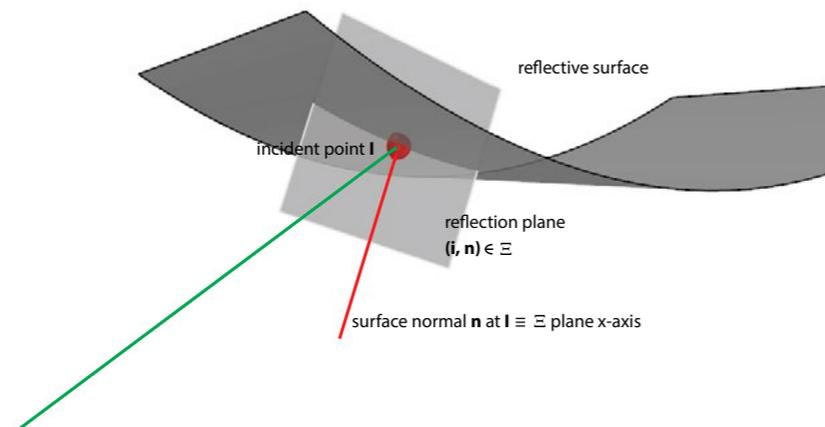
Image 3.35. Geometric definition to describe the reflection of a ray on a surface.
