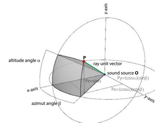
Image 3.33. Geometric parameters for modelling the direction of an acoustic rays by making use of spherical coordinates.
