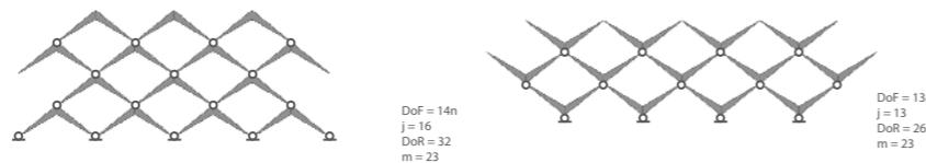
Image 4.17. On plane frame kinematic analysis.
