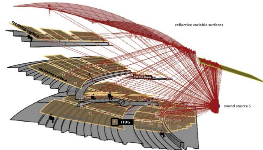
Image 3.38. View of the tool functionality in the Rhinoceros™ digital environment.
