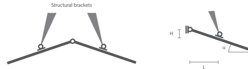
Image 4.25. Kinematic relationships of the folding panels.
