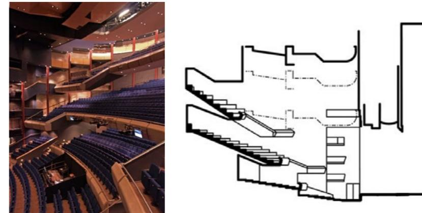
Image 3.20. On the right: long section of the theatre, showing ceiling positions (image courtesy of Barron 2009).
