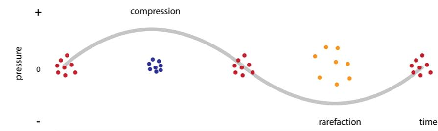
Image 3.1. Full cycle of a continuous sine sound wave in function of time along the x-axis and pressure on the y-axis
