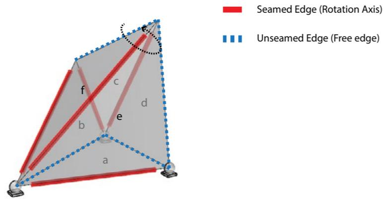
Image 2.42. An irregular bi-pyramid unfolded in a continous strip.
