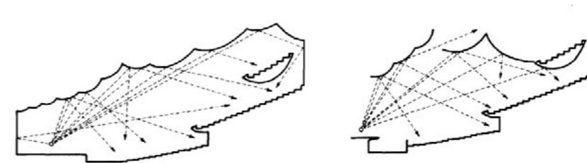
Image 3.17. Edwin Thomas Performing Arts Hall, University of Akron, Ohio. On the left ceiling configuration for concert hall. On the right for opera (image courtesy of Ballou et al 1987).
