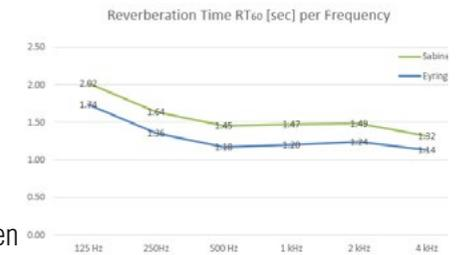
Table 3.4. Output graph of the post-processing excel spreadsheet showing  $RT_{60}$  according to Sabine's and Eyring formulas.
