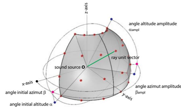
Image 3.34. Sound source implemented with azimuth and altitude amplitude.
