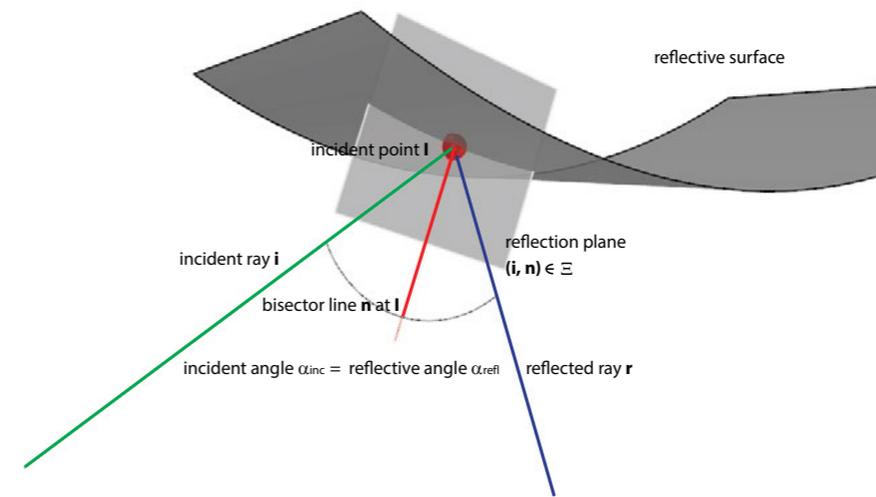
Image 3.36. Calculation by pure geometric consideration of the reflected ray r.
