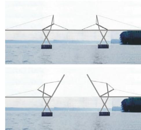
Image 2.18. Concept for a Movable bridge, based on 1D linkages (image courtesy of formfindinglab.princeton.edu).
