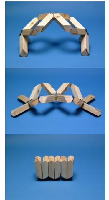
Image 2.24. Network of Bennett linkages (image courtesy of You et al 2012).
