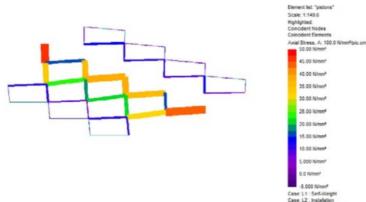
Configuration #1. Max stress 0.41 MPa. Load Case A1.
