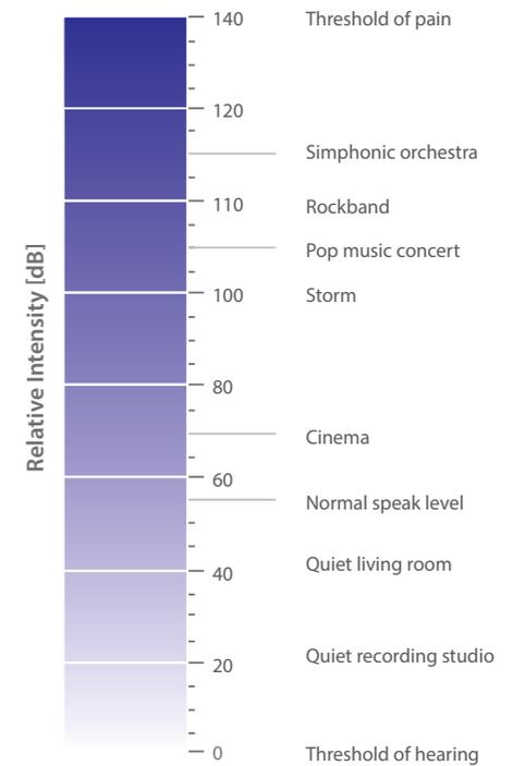
Table 3.1. Comparison of sound pressure and SPL in dB for typical sund sources
