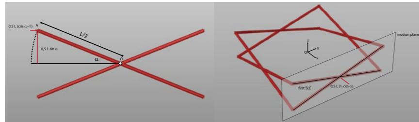
Image 2.23. Left: kinematics of SLE element. Right: motion place for SLE composing a tetrascissor element.
