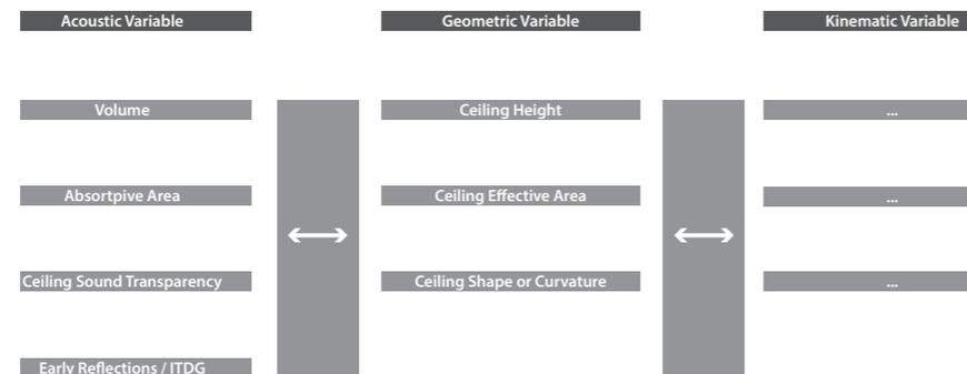
Image 4.01. An abstract framework for the integrate design of the acoustic ceiling.
