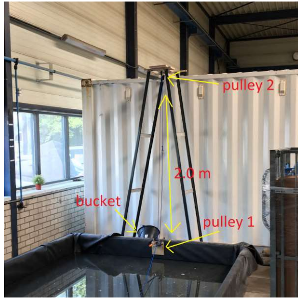
Figure 6.6: tower for fall height
