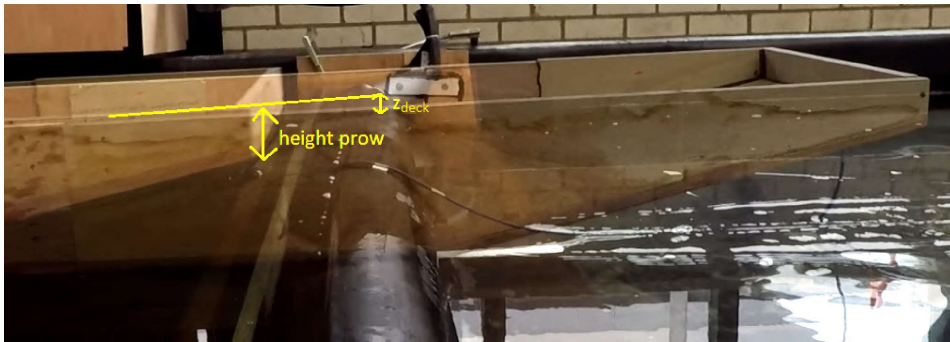
Figure 6.14: displacement measurement ship on weir
