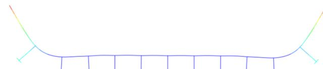
Figure 3:9 Dominant column-like buckling stiffeners side.
