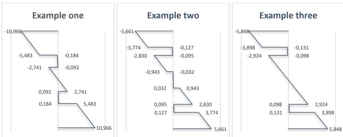
Figure 3.13: Bending stresses in N/mm<sup>2</sup>, according to the Shear analogy
