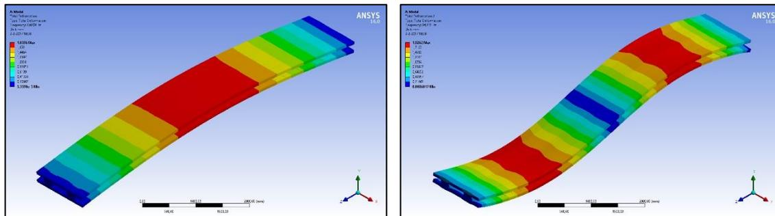
Figure 4.47: First two fundamental frequencies and modal shapes
