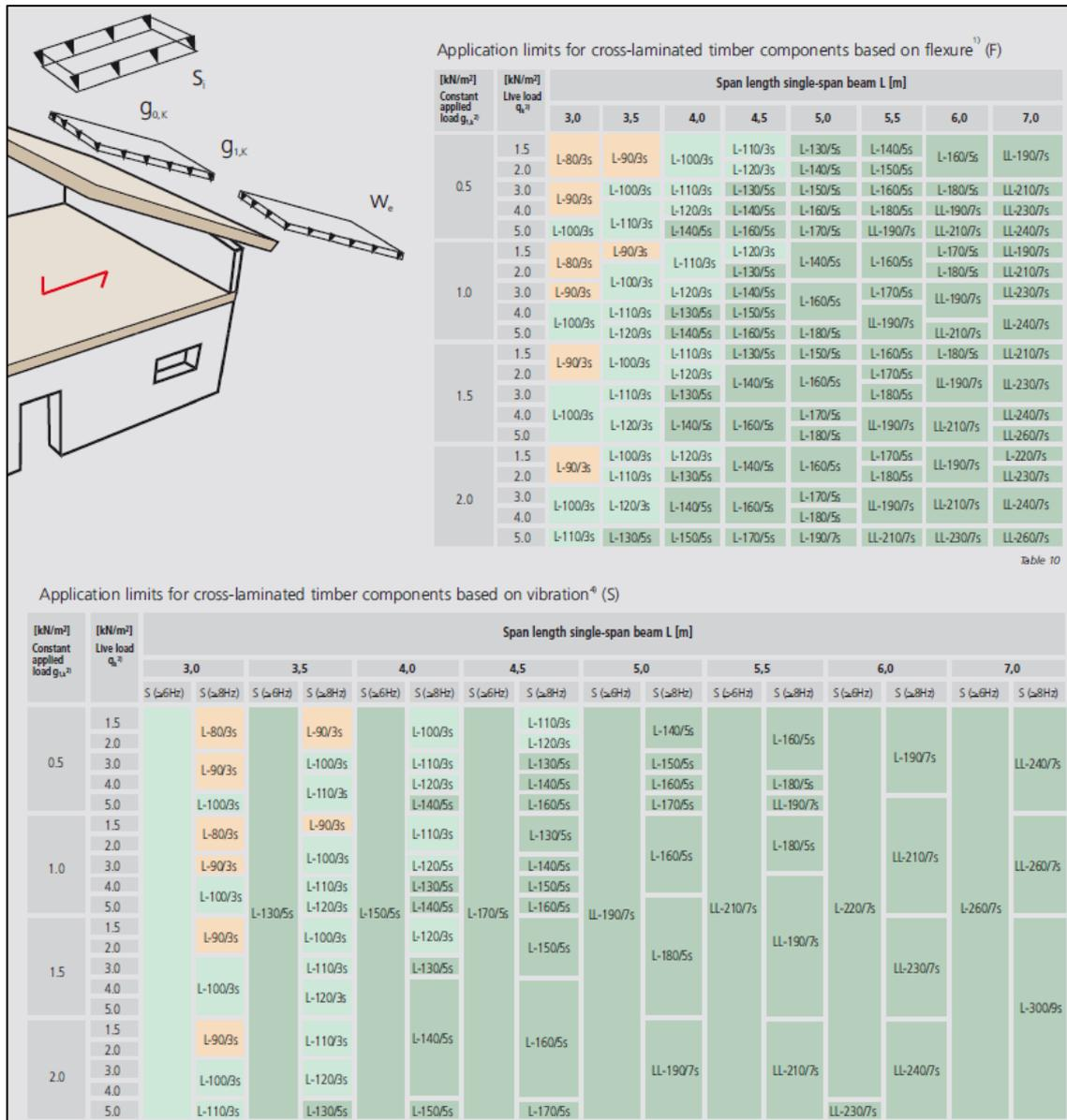
Figure 0.2: Design table - ceiling - single span
