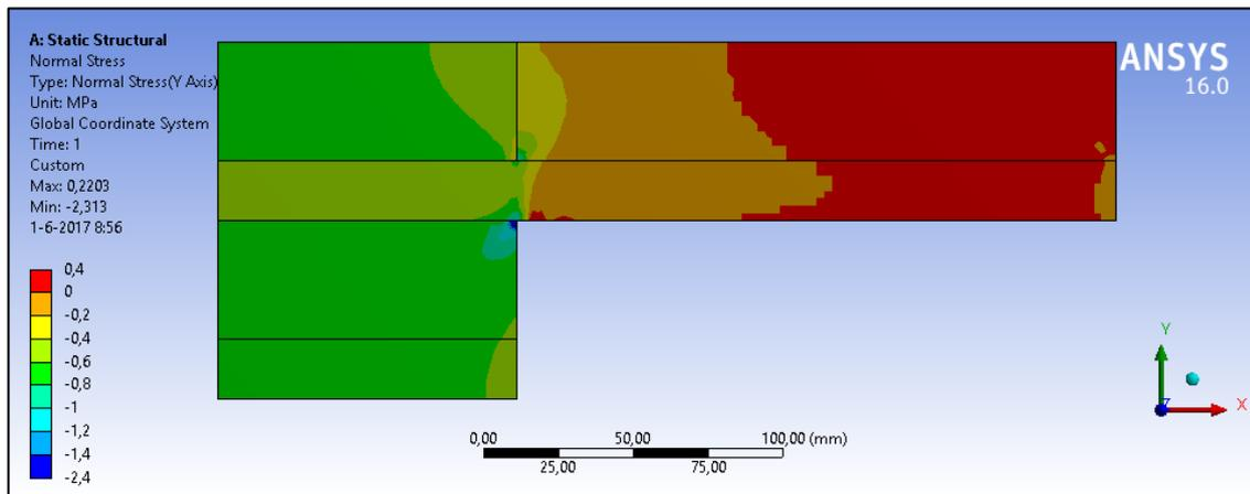
Figure 4.24: Normal stress in y-direction
