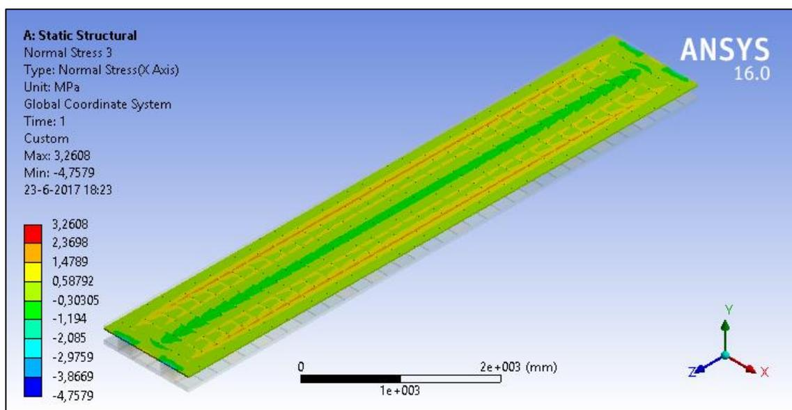
Figure 4.41: Normal stress distribution in x-direction for the top cross layer
