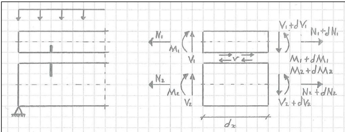
Figure 3.7: System and equilibrium of an incremental element  $dx$
