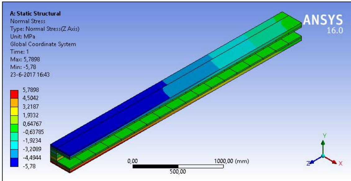
Figure 4.38: Normal stress distribution in z-direction
