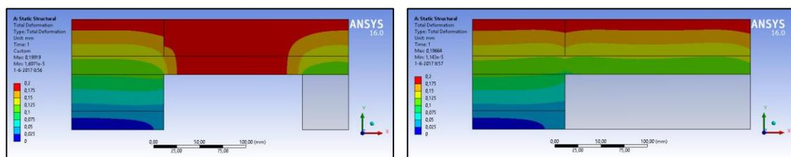
Figure 4.23: Deformation, partially and fully supported
