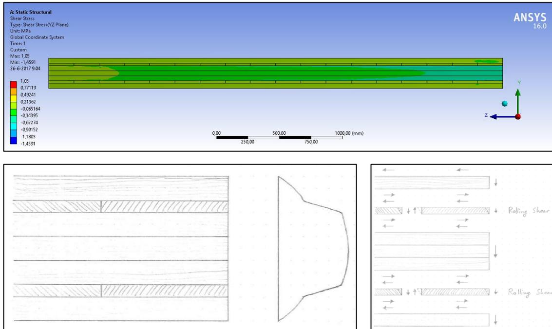
Figure 4.42: Shear stress distribution in the yz-plane
