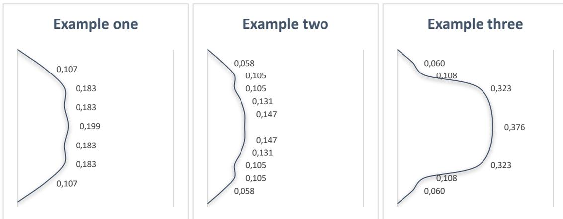
Figure 3.14: Shear stresses in N/mm², according to the Mechanically jointed beams theory
