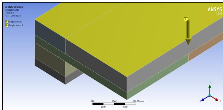
Figure 4.19: Displacement restrictions
