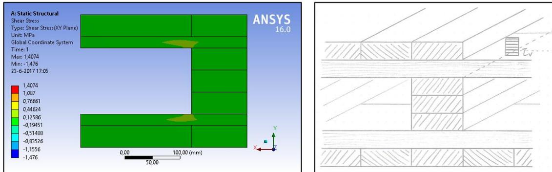
Figure 4.46: Shear stress distribution in the xy-plane
