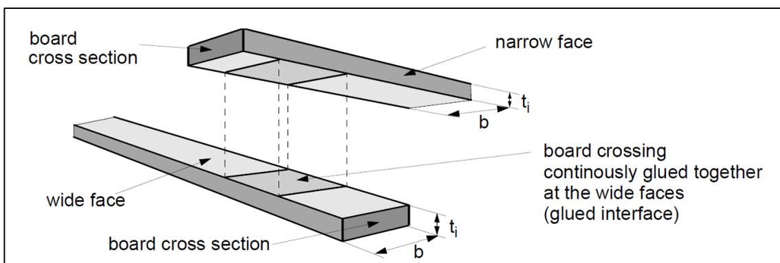
Figure 4.9: Glued joint of a single board crossing
