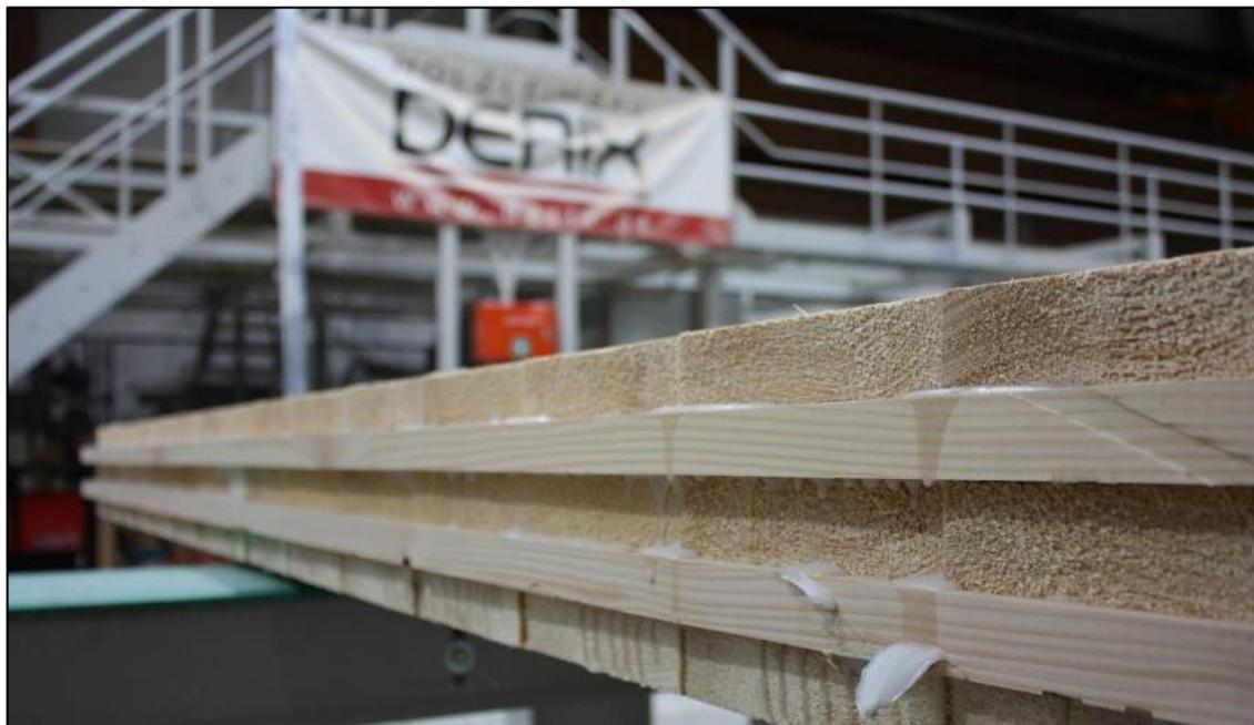
Figure 2.12: Pressed CLT-element, The Derix Group, Niederkrüchten, Germany
