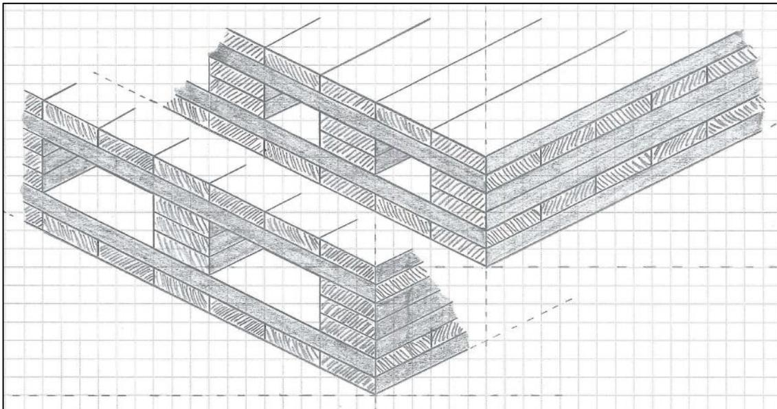
Figure 1.12: Sketch of hollow core cross-laminated timber, two and three layer
