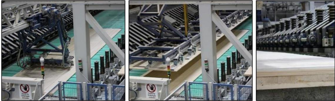
Figure 2.10: Gluing, stacking and pressing of a CLT-element, The Derix Group, Niederkrüchten, Germany
