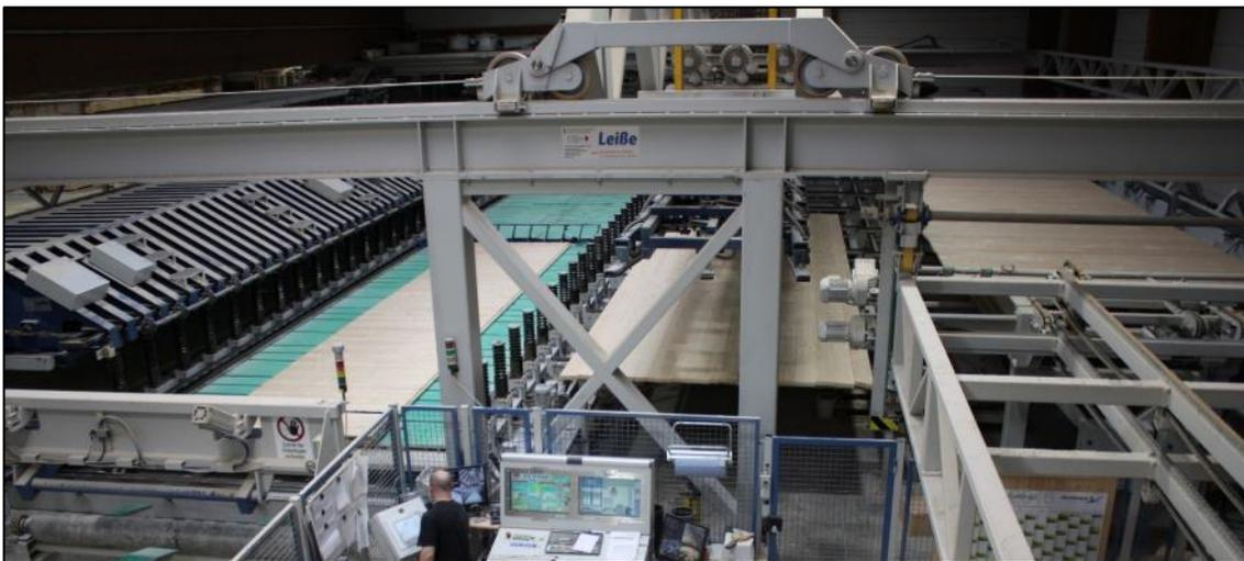
Figure 2.9: Build-up of a CLT-element, The Derix Group, Niederkrüchten, Germany
