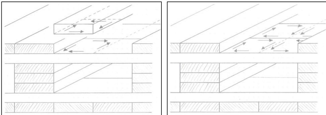
Figure 4.45: Shear resulting in torsion between boards in the flanges
