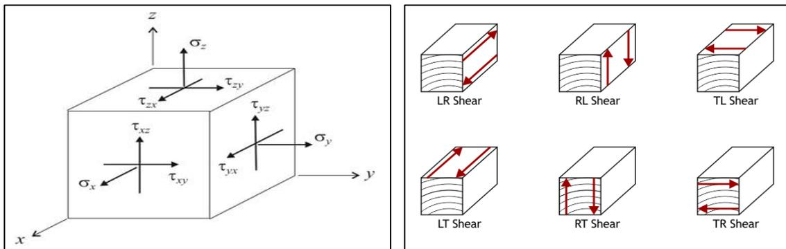
Figure 3.3: Stresses on an element
