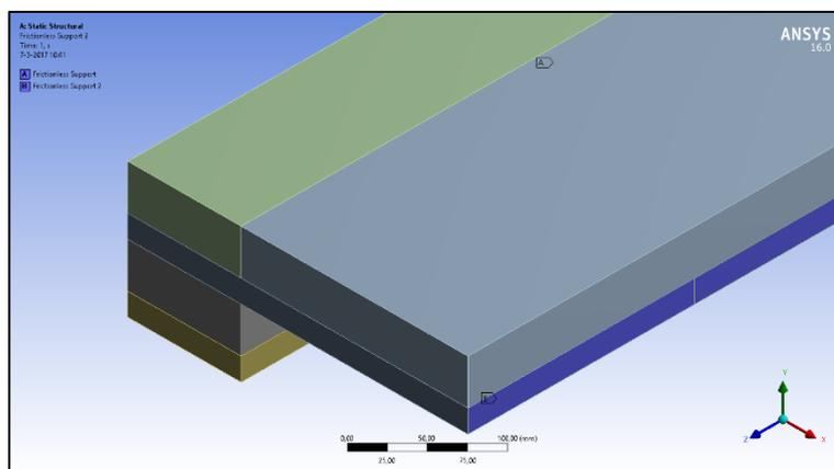
Figure 4.20: Frictionless supports
