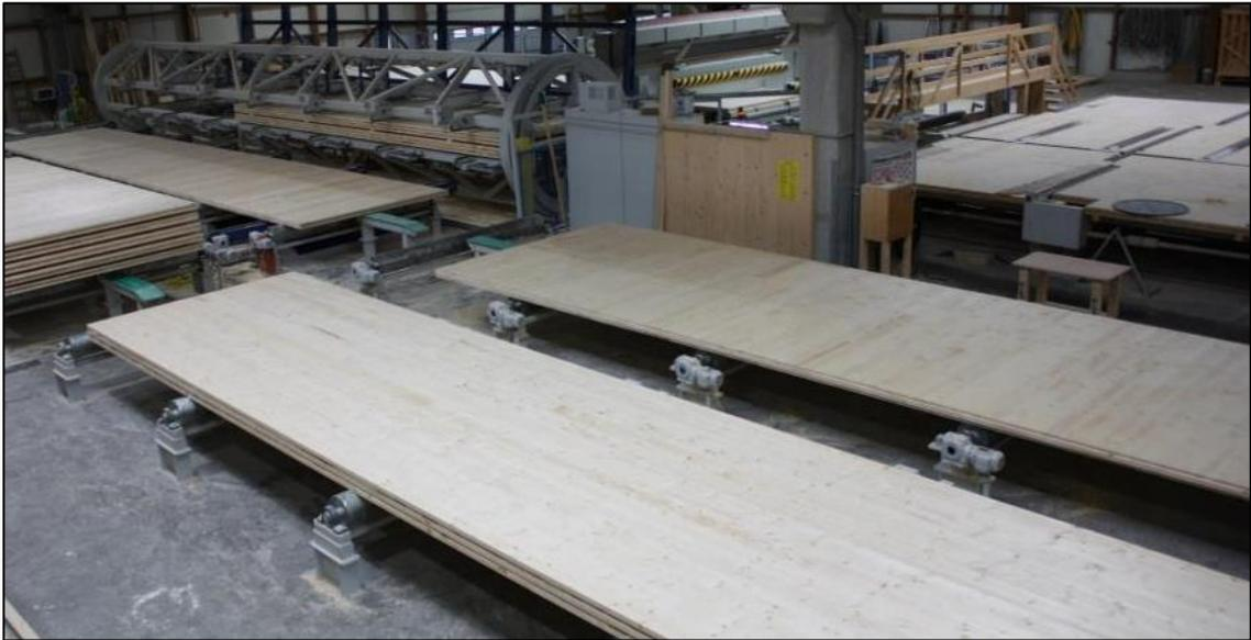
Figure 2.13: CLT-elements and machine for 180 degrees turning, The Derix Group, Niederkrüchten, Germany
