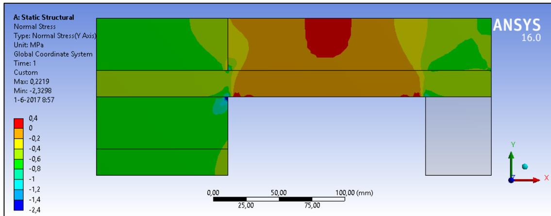
Figure 4.26: Normal stress in y-direction, partially supported
