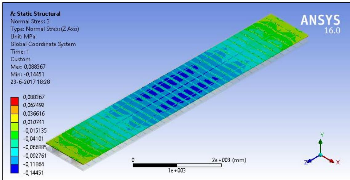
Figure 4.40: Normal stress distribution in z-direction for the top cross layer
