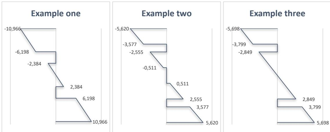
Figure 3.11: Bending stresses in N/mm<sup>2</sup>, according to the Composite method
