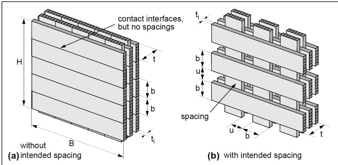
Figure 4.8: CLT without being glued at the narrow faces, with and without intended spacing
