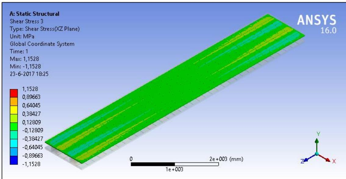
Figure 4.44: Shear stress distribution in the xz-plane for the top cross-layer
