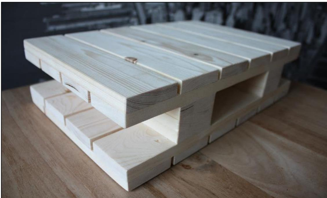
Figure 4.10: HCCLT scale model, non-edge bonded with exaggerated gaps
