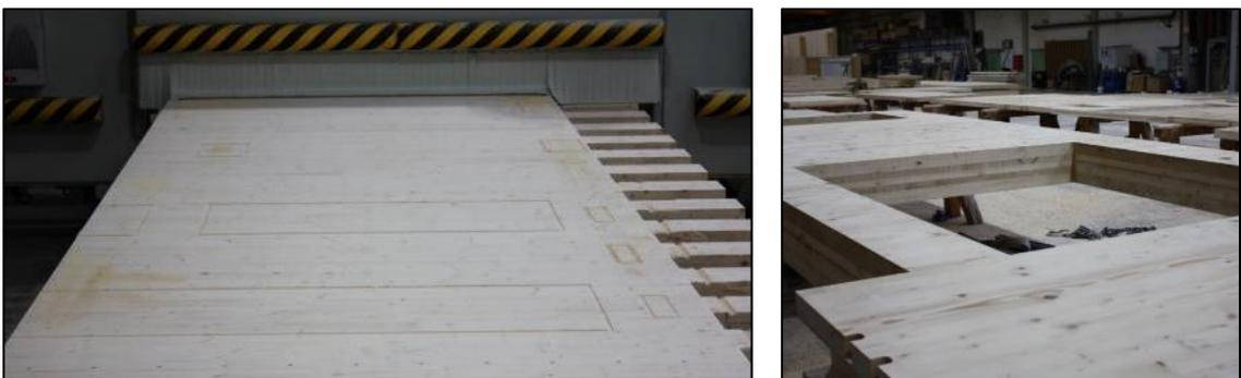
Figure 2.14: CNC-machining and final product, The Derix Group, Niederkrüchten, Germany
