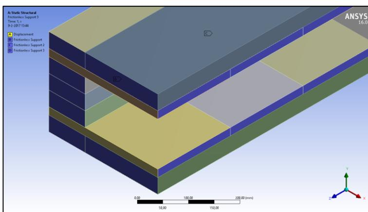
Figure 4.34: Frictionless supports C-profile
