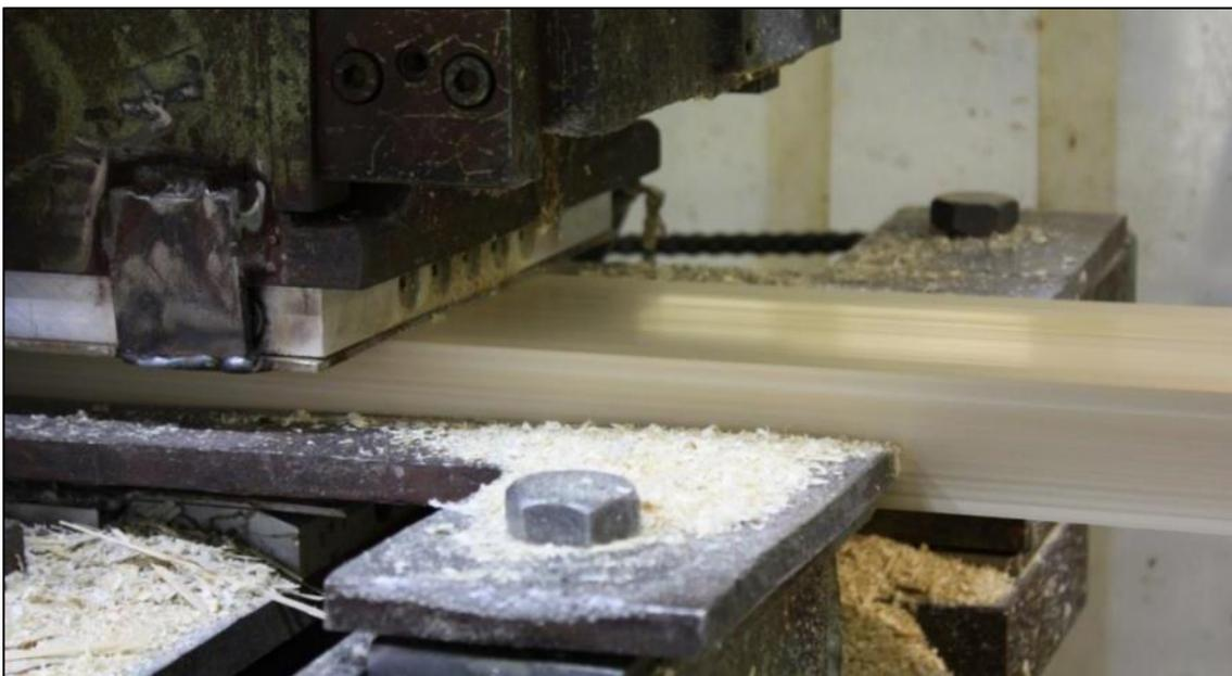
Figure 2.7: Planing and cutting of the "endless" board, The Derix Group, Niederkrüchten, Germany
