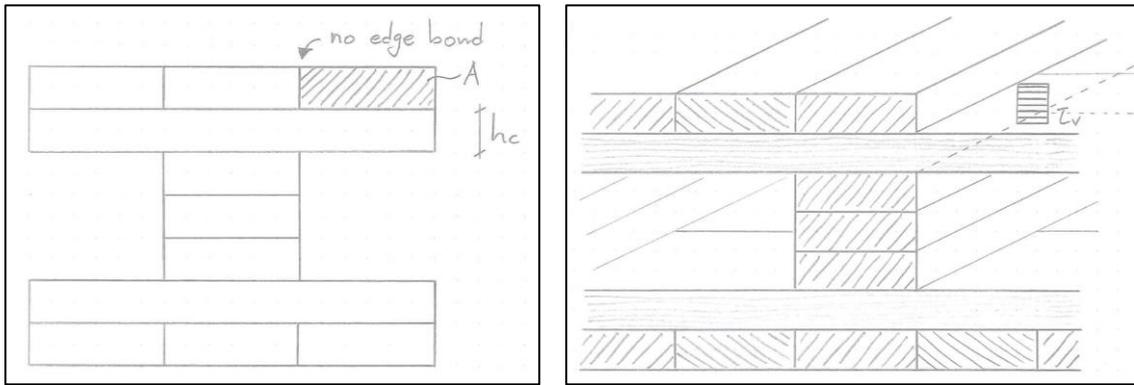
Figure 3.17: Longitudinal shear stress in the cross-layer, due to cooperating flanges
