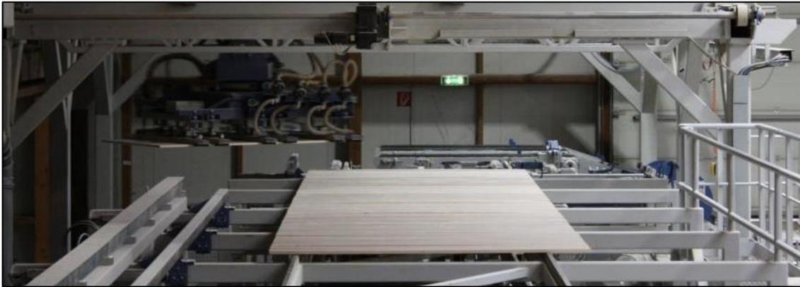
Figure 2.8: Boards for the cross layers, The Derix Group, Niederkrüchten, Germany
