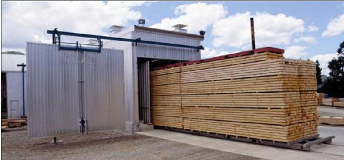
Figure 2.3: Timber Drying Kiln
