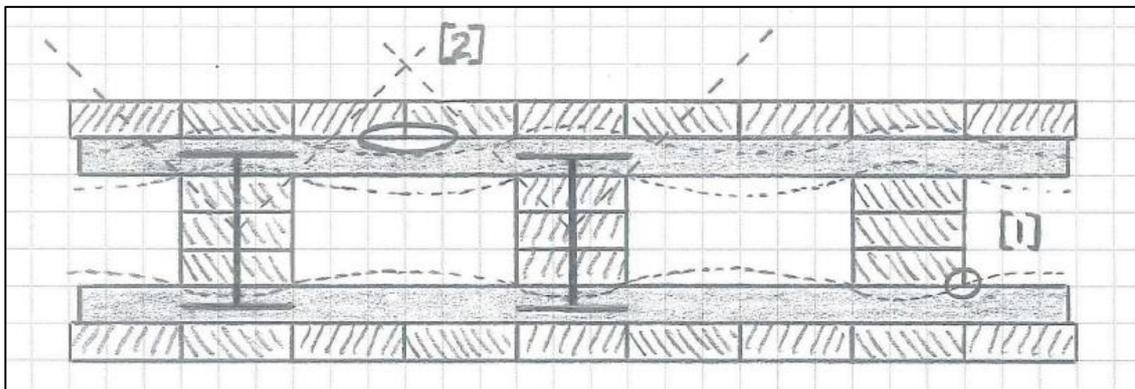
Figure 4.11: Problem areas for manufacturing, Hollow Core Cross-Laminated Timber
