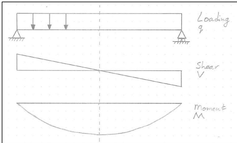
Figure 4.36: Shear & moment distribution, simply supported structure under uniformly loading condition
