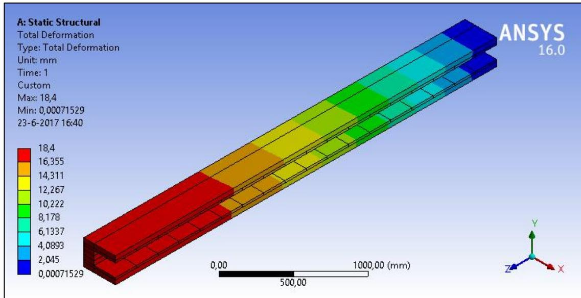
Figure 4.37: Deformation
