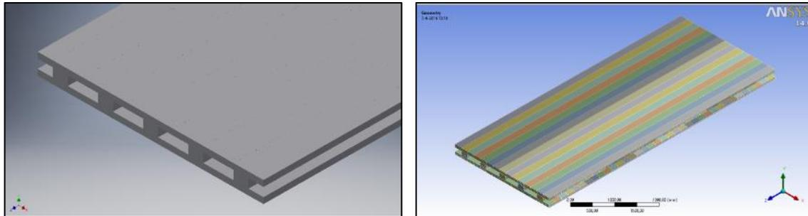
Figure 4.2: “Full” HCCLT-element modelled in Autodesk Inventor
