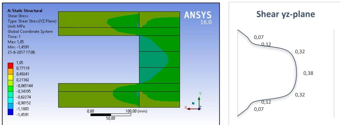
Figure 4.43: Shear stress distribution in the yz-plane
