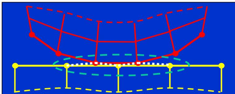
Figure 4.7: Multi-Point Constraint, for bonded contacts only
