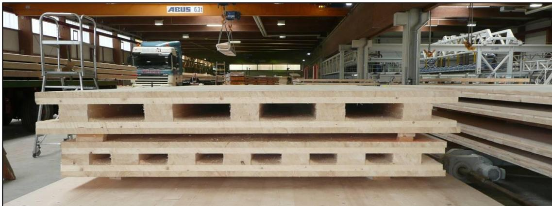
Figure 4.1: Hollow Core CLT-element
