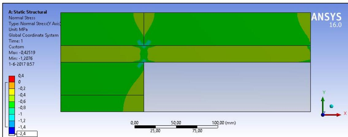
Figure 4.27: Normal stress in y-direction, fully supported
