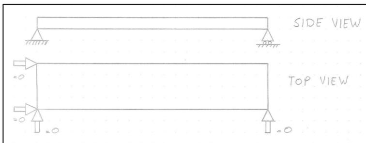
Figure 4.33: Displacement restrictions II-profile
