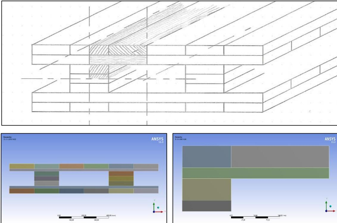
Figure 4.12: Models with an II-profile and, by symmetry, an R-profile
