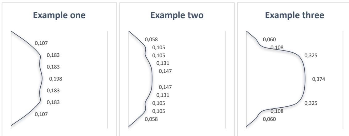
Figure 3.15: Shear stresses in N/mm², according to the Shear analogy
