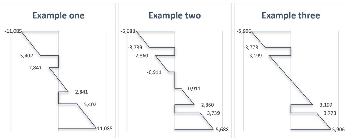
Figure 3.12: Bending stresses in N/mm<sup>2</sup>, according to the Mechanically jointed beams theory
