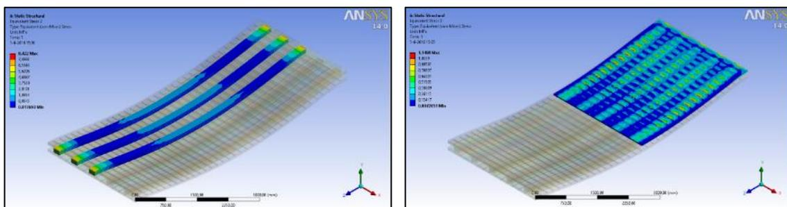
Figure 4.4: Equivalent stress – web and cross layer
