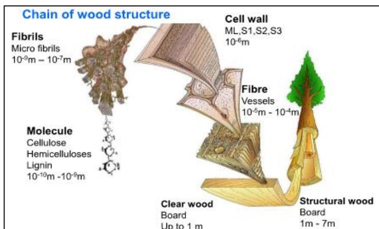
Figure 1.1: Chain of wood structure
