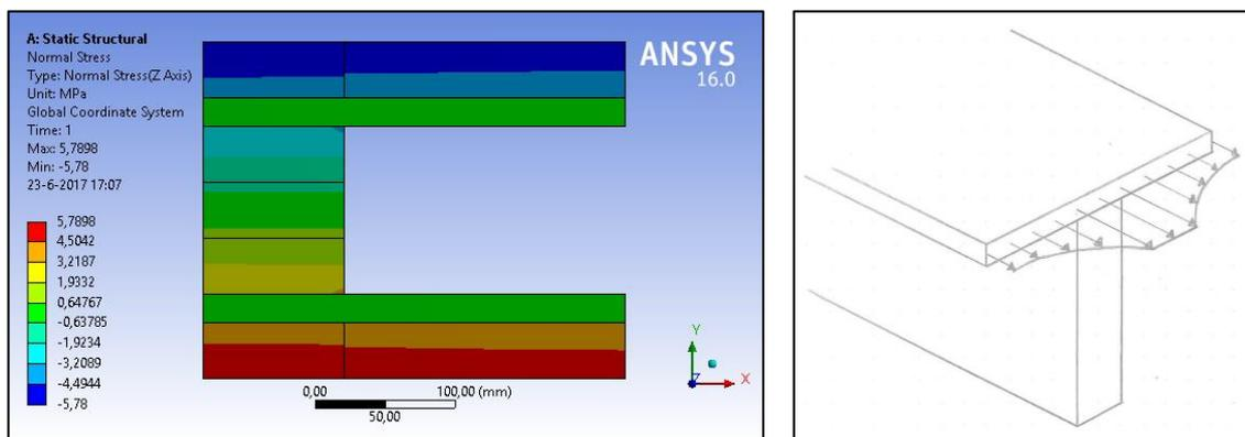
Figure 4.39: Normal stress distribution in z-direction and the effective width of the flange
