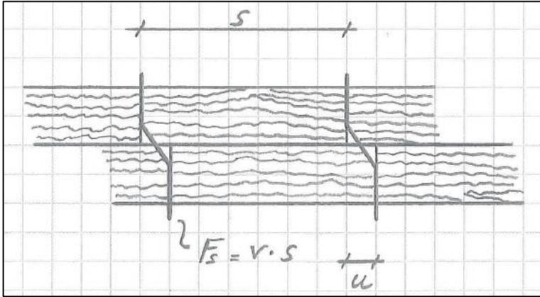
Figure 3.6: Displacement and shear force between the parts
