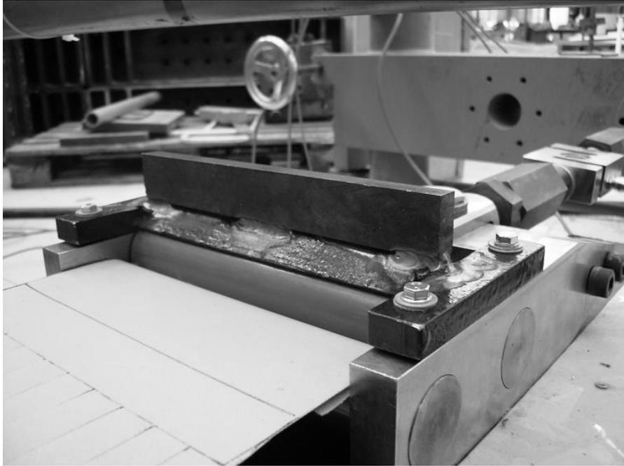
**Figure 94:** Improved bridge with increased stiffness
