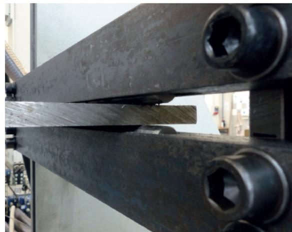
Figure 4.4: Pinned support OSD-specimen[25]
