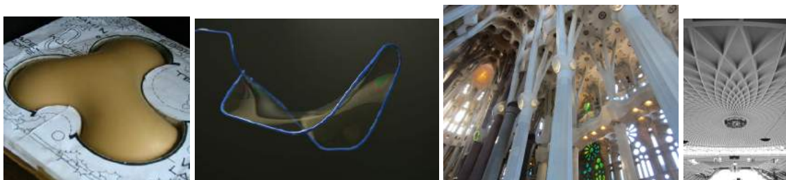
Figure 2.13: (a) pneumatic model, Isler (b) soap film wire loop (c) tree structure, Gaudí (d) ribbed shell, Nervi
