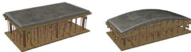
Figure 2.27: (a) Plate mould, horizontal casting position (b) deformed plate mould
