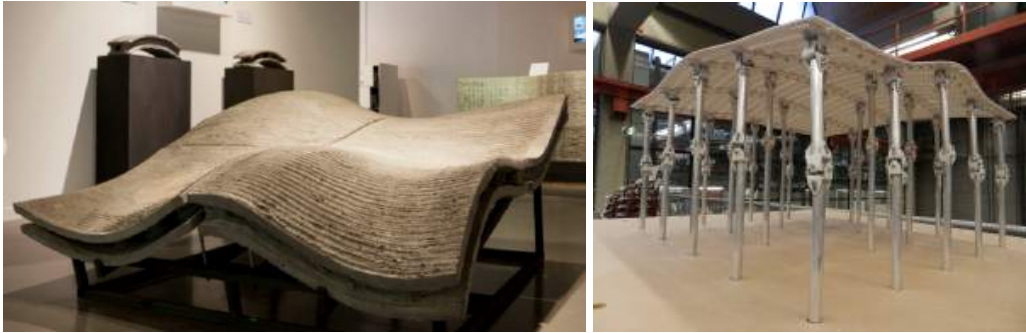
Figure 2.21: (a) 3d-Printed double curved concrete elements (b) Flexible formwork [25]
