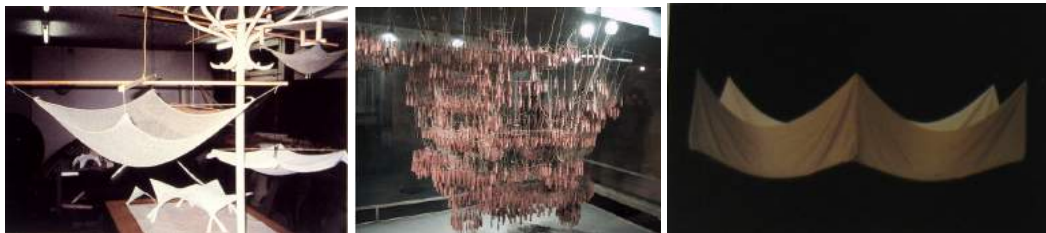
Figure 2.12: (a) hanging models Isler (b) hanging sandbags in model Gaudí (c) wrinkling hanging membrane
