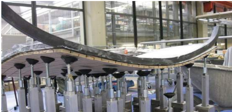
Figure 2.24: Adjustable mould used by Huyghe and Schoofs [19]
