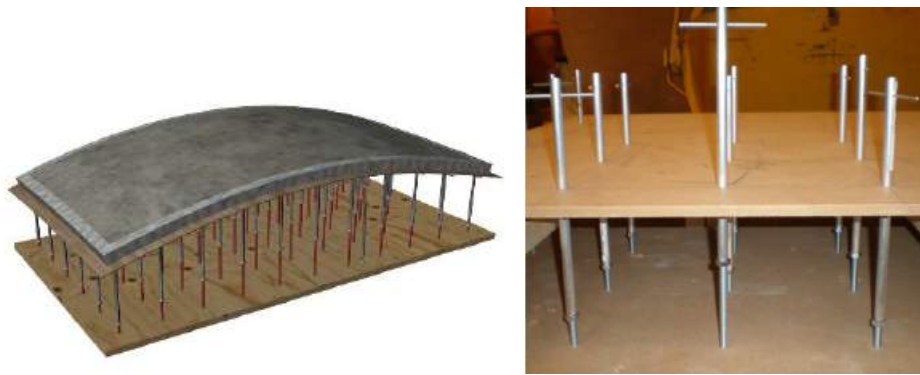
Figure 2.25: (a) Adjustable formwork (b) Actuators
